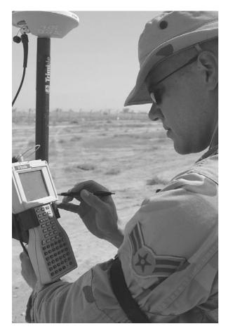
Global Positioning System (GPS) technology uses multiple communication satellites to allow military forces to determine more precisely their position—and that of their enemies. Here a U.S. Air Force airman uses a handheld GPS device to conduct a data collection survey in Iraq in 2004. (Department of Defense)
