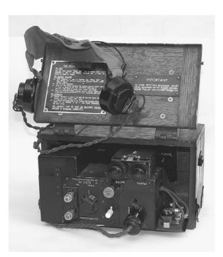
The Fullerphone was, despite its name, a system of portable line telegraphy developed in the British army signals service in 1915. It transmitted over telephone lines without interfering with those signals and was difficult to overhear, making it ideal for the static trench warfare of the Western Front in World War I. (Courtesy Louis Meulstee)
