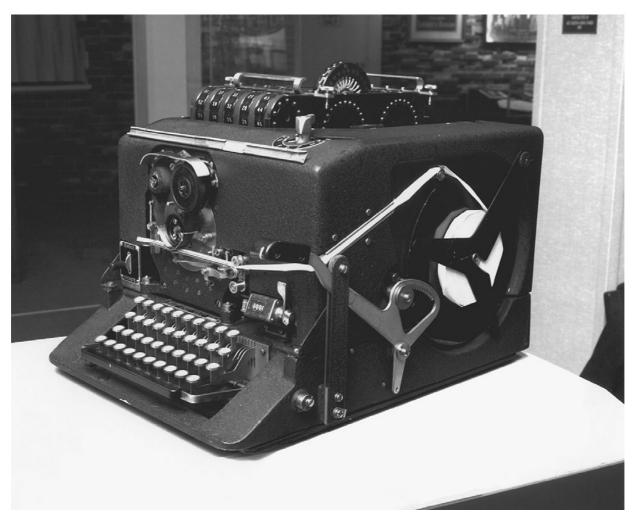
*Officially the Electric Cipher Machine (ECM), the complex SIGABA became the mainstay American ciphering device used in World War II. Its signals were never broken by Axis enemy forces. (National Security Agency)*
