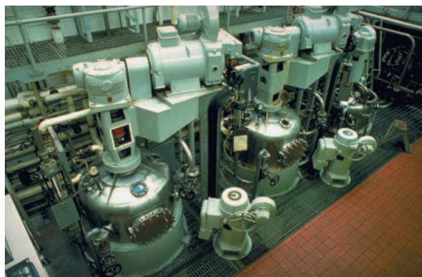
Commercial fermentation units like these are used to grow cultures of microorganisms for biological products like interferon. Photograph by S. Stammens. National Audubon Society Collection/Photo Researchers, Inc. Reproduced by permission.
