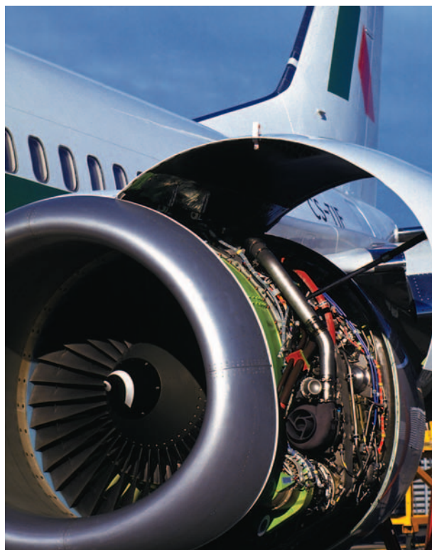
A jet aircraft with the engine cover open. The engine works by sucking air into one end, compressing it, mixing it with fuel and burning it in the combustion chamber, and then expelling it with great force out the exhaust system. Photograph by George Haling. Photo Researchers, Inc. Reproduced by permission.
