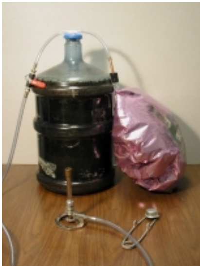
Completed biogas generator.
