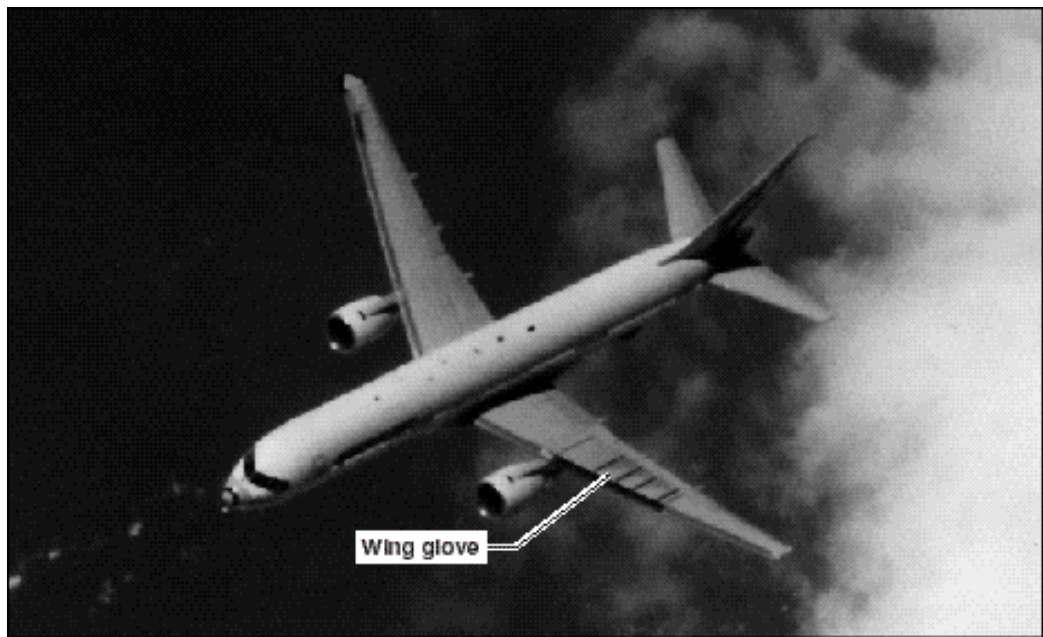
Figure 18. 757 subsonic hybrid laminar flow control flight experiment. (NASA photo L-90-9549)
