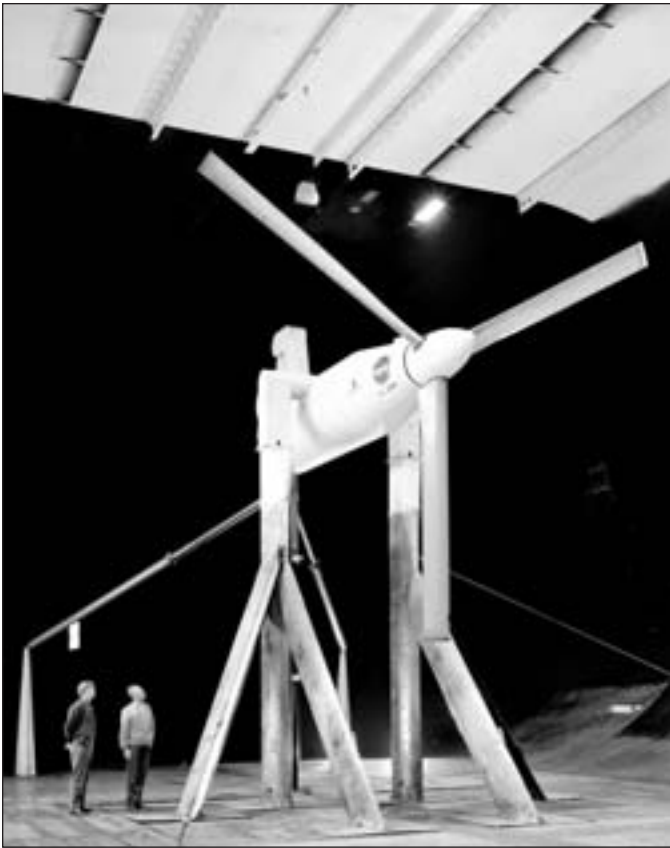
Figure 31. Bell 25-ft. diameter proprotor performance test in the Ames Research Center 40- by 80-ft. wind tunnel. (Ames Photograph AC70-5390)
