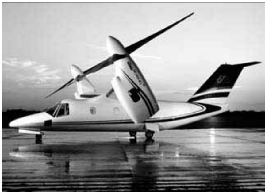
Figure 77. Mockup of the BA-Model 609 civil tilt rotor aircraft with Bell-Boeing markings. (Bell-Ames Photograph ACD97-0133-3)
