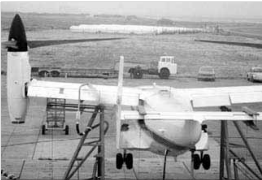
Top: Figure 56. Flow visualization near the XV-15 wing tips. (Ames Photograph AC85-0804-49)
