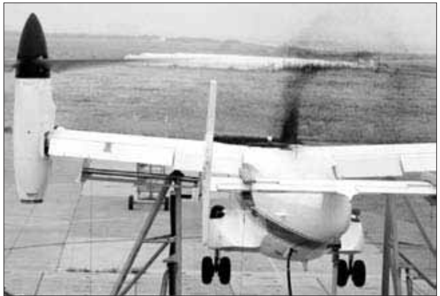
Figure 58. Inboard flow visualization showing "fountain flow" above fuselage. (Ames Photograph ACD-0804-3.1)
