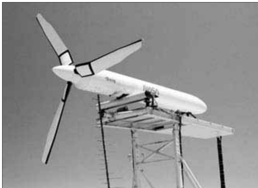
Figure 63. Advanced Technology Blades proprotor mounted on the test apparatus at the Ames Research Center Outdoor Aerodynamic Research Facility. (Ames Photograph AC84-0498-2)
