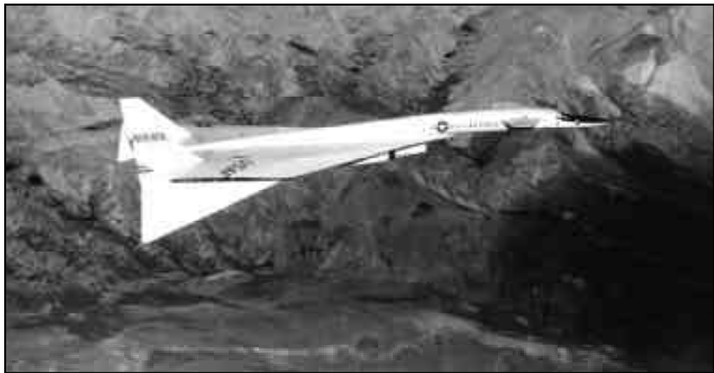
In this photo the Number 1 XB-70A (62-0001) is viewed from above in cruise configuration with the wing tips drooped for improved controllability. (NASA photo EC68-2131)
