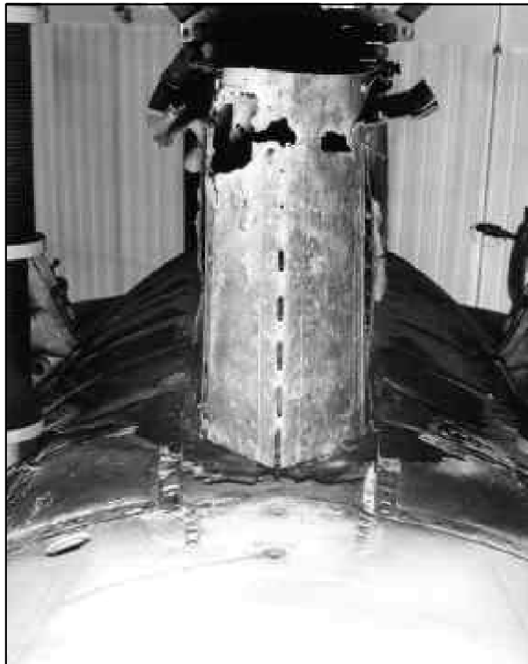
Figure 14: Result of severe heating from the Mach 6.7 flight in the X-15A-2. (NASA photo E-17525)
