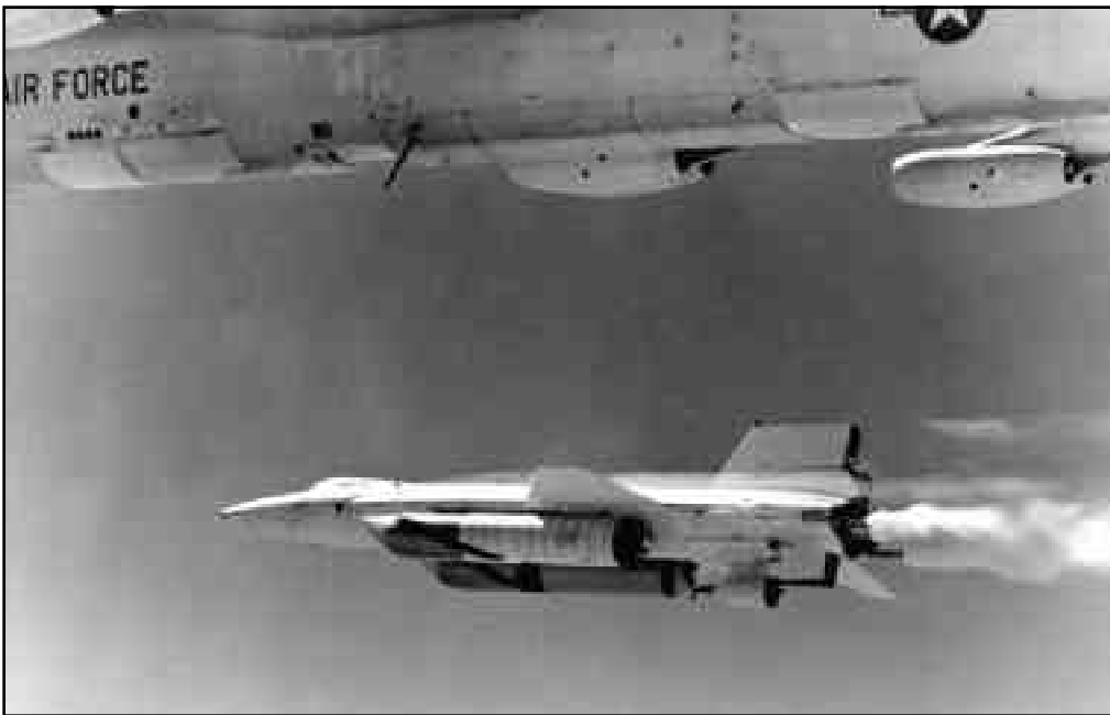
Figure 13: Photo showing X-15A-2 with ablative coating, drop tanks, and dummy ramjet. (NASA photo ECN 1889)
