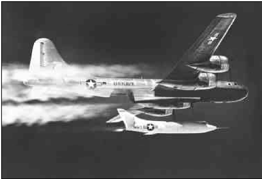
The D-558-2 Number 2 is launched from the P2B-1 in this 1956 NACA High-Speed Flight Station photograph. This is the same airplane that Scott Crossfield had flown to Mach 2.005 in 1953. (NASA photo E-2478)
