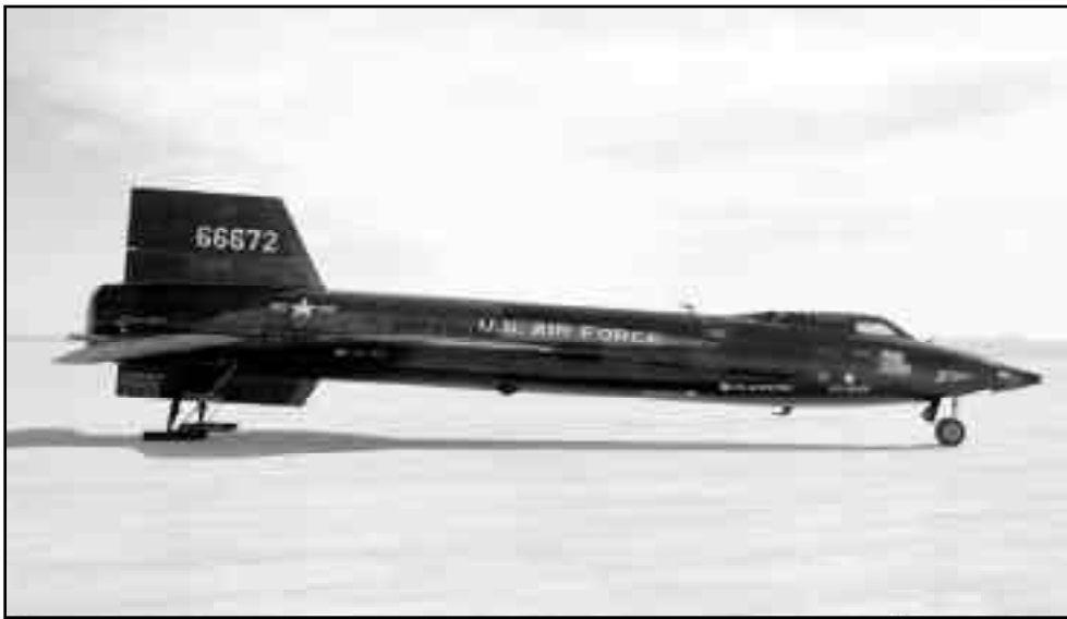
The X-15 ship Number 3 (56-6672) is seen here on the tarmac at the Edwards Air Force Base, California. Ship Number 3 made 65 flights during the program, attaining a top speed of Mach 5.65 and a maximum altitude of 354,200 feet. (NASA photo E-7896)
