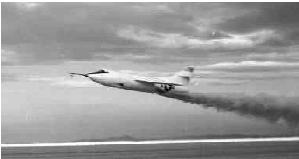
A Douglas D-558-II Skyrocket taking off from the lakebed. Completely different from the jet-powered, straight winged Skystreak, the Skyrocket featured swept wings and a variety of propulsion systems. Flying a Skyrocket, NACA research pilot Scott Crossfield became the first to fly faster than Mach 2. (E49-219)
