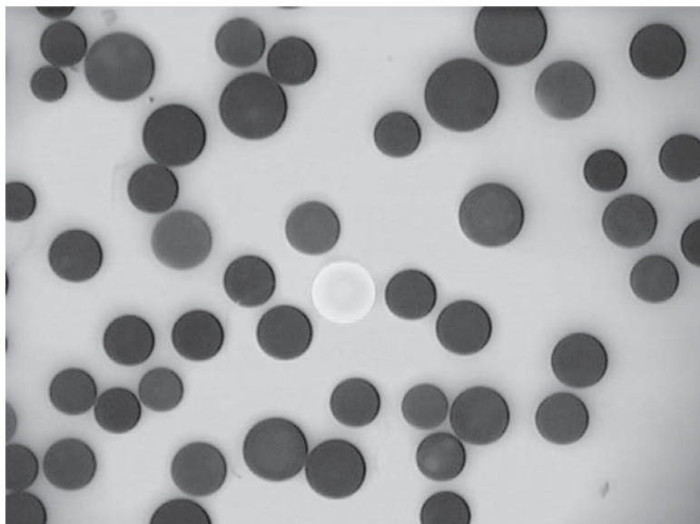
Fig. 3. Fluorescent photomicrograph of beads revealing one fluorescent bead (near the center of the field) obtained after digestion of its peptide had released the quenching Dabsyl moiety.
