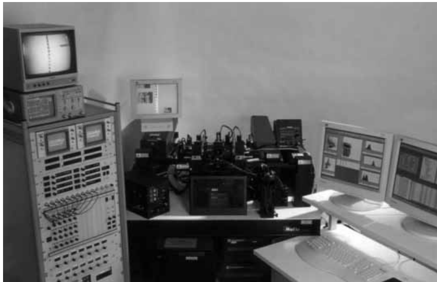
Fig. 9.1. A sorting flow cytometer (MoFlo by Cytomation). The outward complexity of this instrument compared with benchtop cytometers (see Fig. 1.5) reflects the electronic controls necessary for sorting as well as the adaptability of research cytometers with regard to multiple lasers and to the filters and mirrors in the optical light path for multiparameter analysis.
