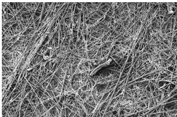
Fig. 1 Random depth filter matrix (courtesy of Sartorius Group)
