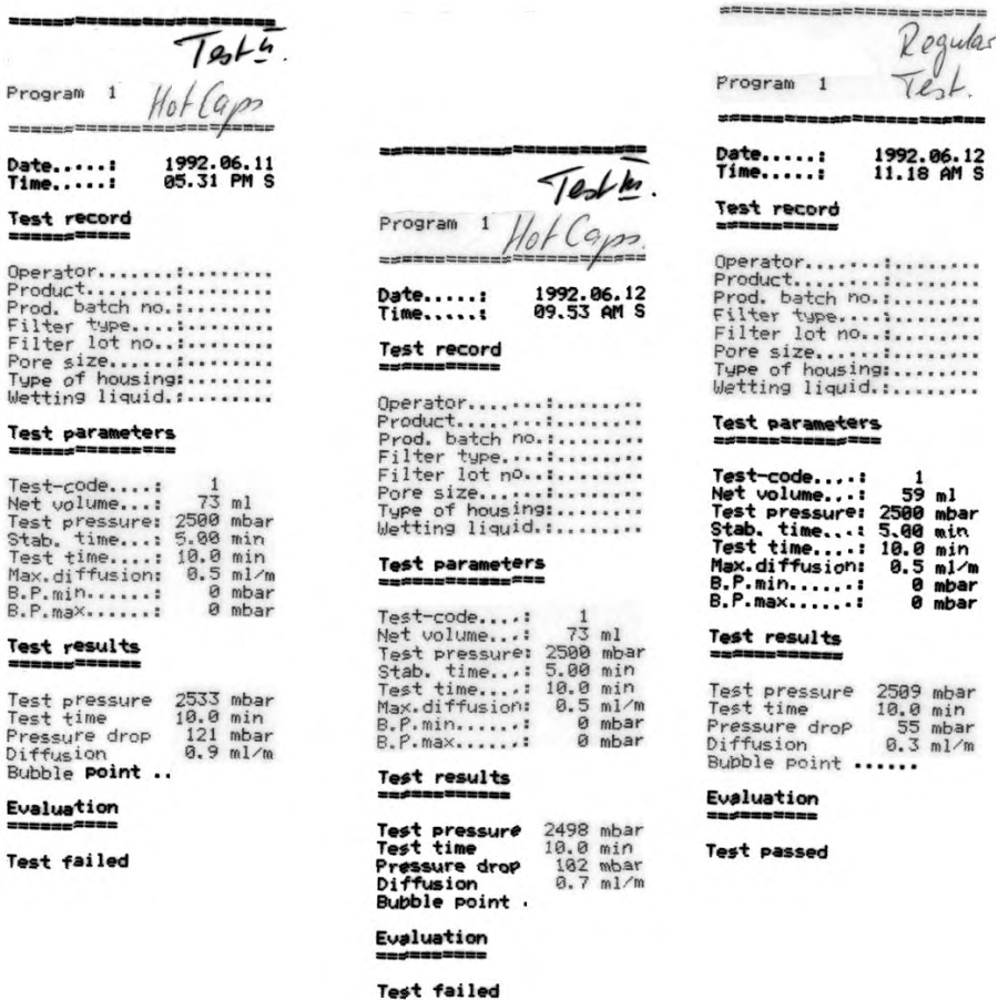
Fig. 6 Examples of test failures due to temperature differences
