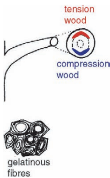
Figure 3.6. Reaction and tension wood (gelatinous fibres detailed).
