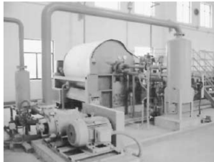
Figure 3.115 (a) Schematic diagram of a rotary vacuum filtration system. (b) Photograph of a large vacuum filtration system. (Courtesy of WesTech Engineering.) (c) Photograph of a small custom-built vacuum filtration system. (Courtesy of EIMCO Process Equipment Co.)
