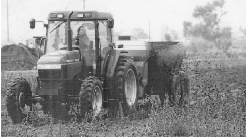
Figure 7.6 Surface application of dewatered biosolids. (Courtesy of Leland Myers, Central Davis Wastewater Treatment Plant, Kaysville, Utah.)
