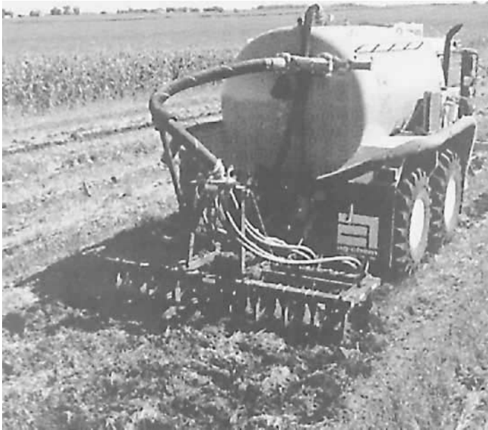
Figure 1.7 Soil injection of biosolids used to comply with the 40 CFR Part 503 vector attraction reduction requirements.
