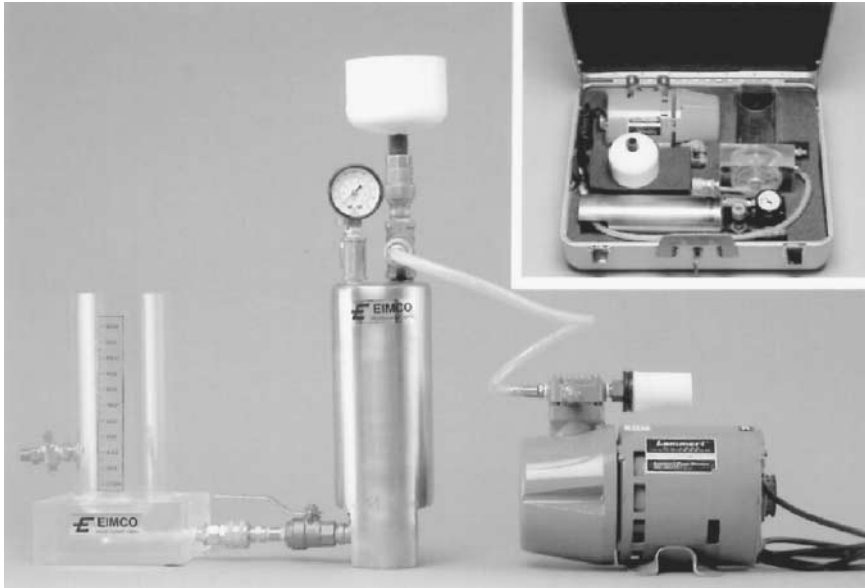
Figure 3.12 Bench scale system to estimate air-to-solids (A/S) ratio. (Courtesy of EIMCO Process Equipment Co.)
