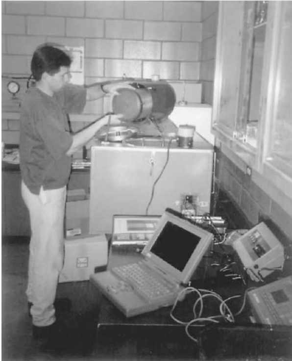
Figure 3.76 A technician evaluating various compost mixtures using a laboratory scale compost system. (Courtesy of Cache Environmental Laboratory, P.C.)
