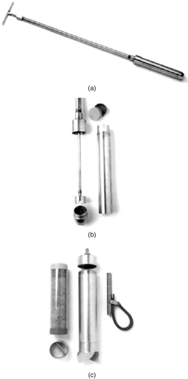
Figure 8.4 Photographs of coring devices for sampling dewatered sludge/biosolids: (a) discrete sludge sampler to obtain sludge/biosolids at desired depth; (b) slotted piston for discrete sludge sampler; (c) core sludge sampler equipped with one-way valve. (Courtesy of Art's Manufacturing & Supply, Inc.)
