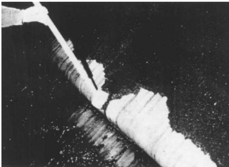
Figure 8.1 Photograph of a wastewater treatment operator taking a dewatered biosolids/sludge sample. (Courtesy of the Water Environment Federation.)
