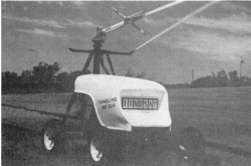
Figure 7.8 Photograph of a traveling-gun biosolids sprayer.
