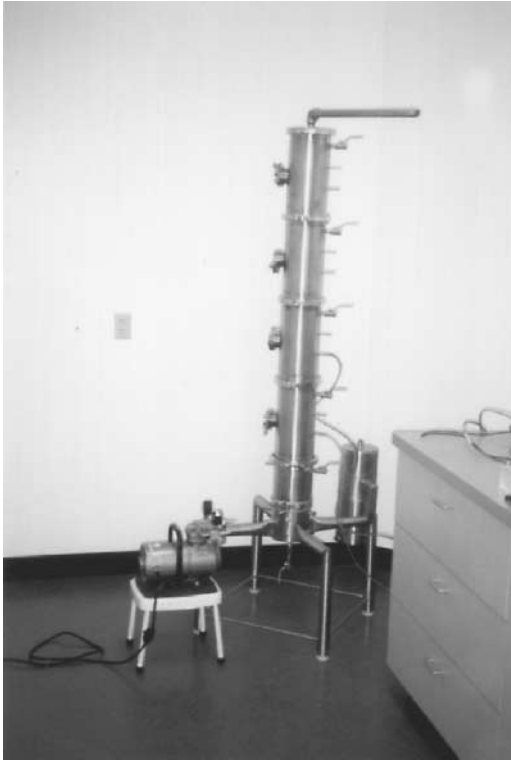
Figure 5.91 Photograph of a laboratory-scale soil/compost filter bed used to evaluate full-scale design parameters. (Courtesy of Cache Environmental Laboratory, P.C.)
