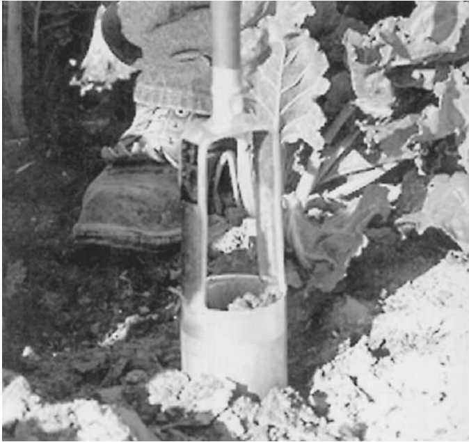
Figure 8.7 Photograph of a soil sample taken from an agricultural field using an auger. (Courtesy of Art's Manufacturing and Supply, Inc.)
