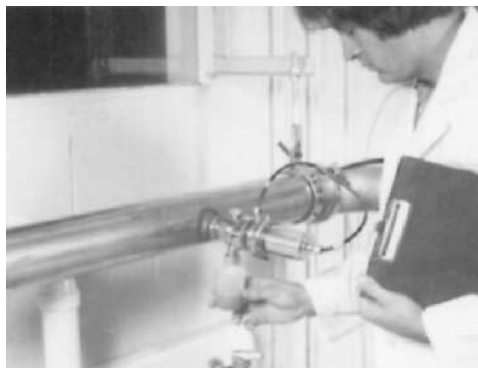
Figure 8.2 Photograph of an automatic sampling device for use in pressurized sludge/biosolids pipelines. (Courtesy of Bristol Equipment Company.)
