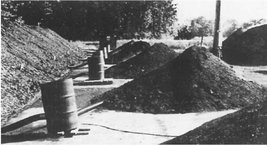
Figure 3.82 Odor control piles for aerated static pile compost system.
