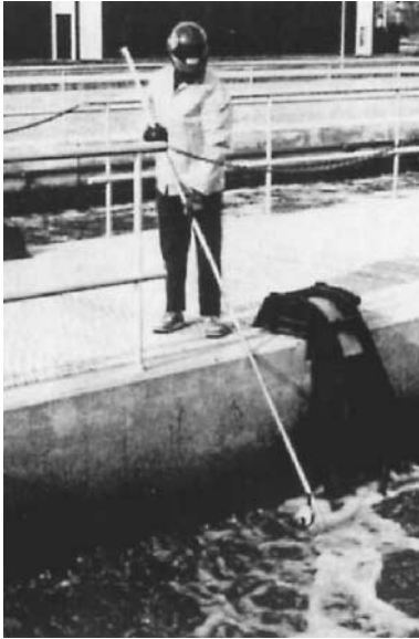
Figure 8.3 Photograph of a pond sampling device for unpressurized sludge/biosolids sampling. (Courtesy of the Water Environment Federation.)
