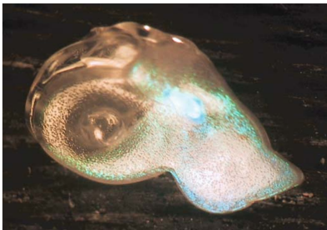
FIGURE 12.2. Poly(lactide) molded from a porous Si photonic crystal template. This polymer contains the drug caffeine. Decay of the optical spectrum (the green color visible in the image) from this fixture provides a surrogate measure of the drug delivery rate.
