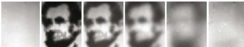
FIGURE 17.2. Fluorescence recovery after photobleaching (FRAP) experiment on a supported membrane. First panel: Initially uniform fluorescence from the yet unbleached membrane. Second panel: Bleach pattern shortly after exposure. Subsequent panels: Time sequence of images illustrating diffusive mixing of the bleach pattern with nearby unbleached regions of membrane. Adapted from [80].
