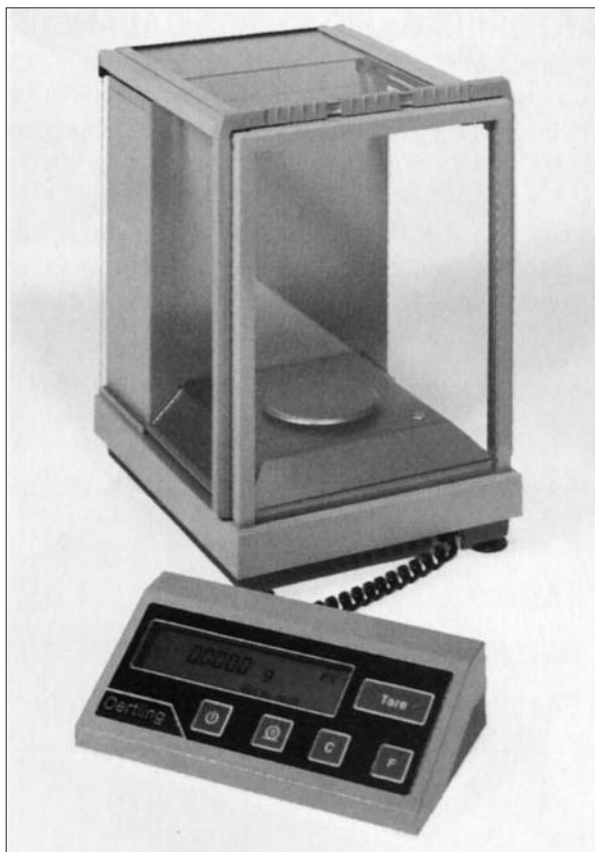
A laboratory balance. This balance measures masses as low as 0.0001 g.
