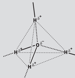
Fig. 5.16 Hydrogen bonding in water. Note that the O···H bonds are longer and weaker than the O–H bonds.
