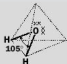
Fig. 5.2 The structure of the water molecule.
