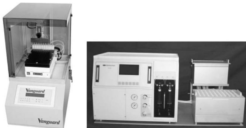
Fig. 6 Semi-automated synthesizers: aapptech Vanguard (left) and MultiSynTech SAS (right).
