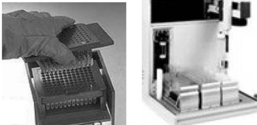
Fig. 10 Phase separation using Radleys' "Lollipop" method (left) and the fully automated Mettler Toledo ALLEXis (right).
