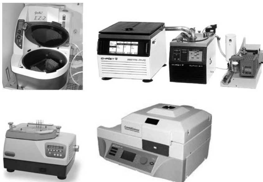
Fig. 11 High-throughput vacuum evaporators: Genevac EZ-2 and Christ Beta-RVC centrifuges and Labconco and Hettlab CombiDancer shakers.
