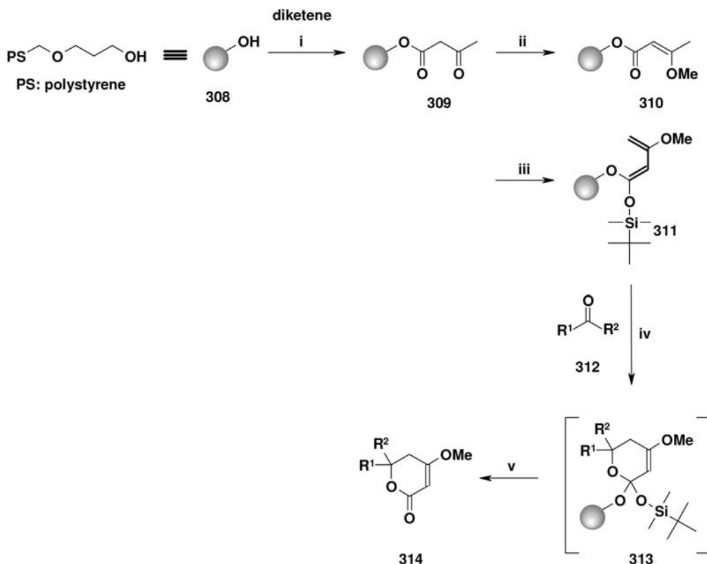
Scheme 66 (i) Diketene, DMAP, CH 2 Cl 2 , -50 °C, r.t.; (ii) TMOF, H 2 SO 4 cat., then heating at 60 °C; (iii) (a) LDA, THF, -78 °C, then r.t., (b) DMPU, TBDMSiCl, -78 °C, then r.t.; (iv) Me 2 AlCl, -78 °C to r.t.
