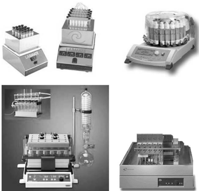
Fig. 5 Manual synthesizers: aapptech LABMATE, Heidolph Synthesis 1, Chemspeed MSW 500, and Büchi Syncore (clockwise from top left).
