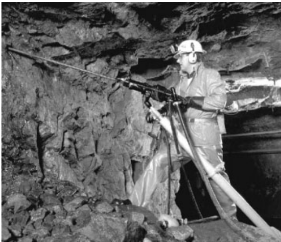
Figure 39.6 One man–one machine, a drilling technique in diamond mines. (Reprinted with permission of Atlas Copco Rock Drills AB, Sweden.)
