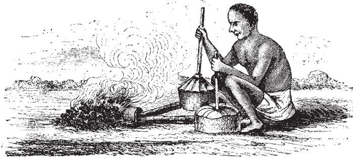
Figure 8.12 A village inhabitant in Simarianjo operates two bellows at the iron furnace. (A drawing by David Livingstone, reprinted from ref. [8.9].)
