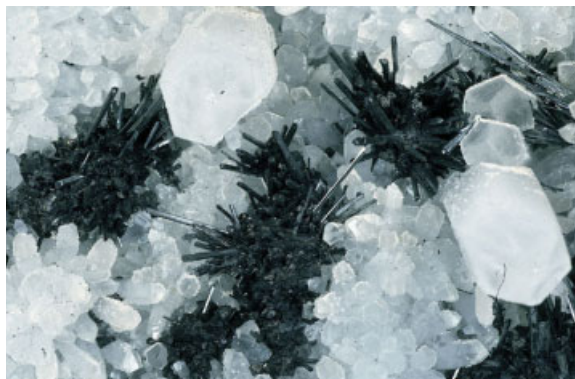
M72 Stibnite, antimony glance, Sb_2S_3 , orthorhombic crystals, black shining, like a spear (Latin stibnium ), and crystals of quartz. Collected by Kay Sund in the 200 me- ters level in the Baia Mare mine in Romania.
