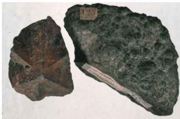
M76 Uraninite \text{UO}_2 to the left. A cubic twin crystal from Stackebo in the Province of Älvsborg in southern Sweden. Pitchblende \text{UO}_2 to the right, from Joachimsthal in Erzgebirge, Germany
