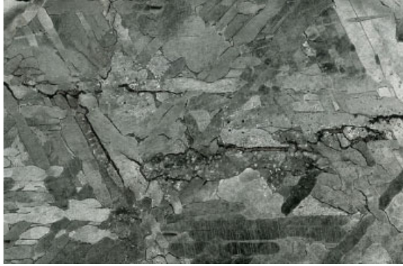
M7 Meteorite iron with Widmanstätten structure, found in Xiquipilco, the Toluca region in Mexico.
