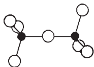
Figure 40.4 A sorosilicate ion. The silicon atom to the left “owns” alone the three oxygen atoms to the left and has a half share in the middle oxygen atom. This implies that every silicon atom binds on average to 3.5 oxygen atoms; O/Si=3.5 .
