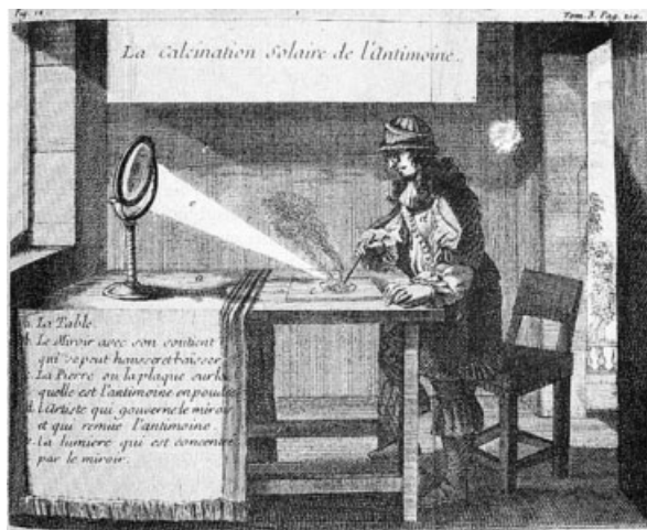
Figure 46.2 Heating with a burning glass was utilized in early chemistry. This picture, from LeFevre, Cours de Chymie , shows calcination of an antimony mineral.
