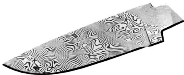
Figure 8.19 Blade of a knife made from a twisted bar of damask and etched. (Reprinted with permission from P. and M. Billgren, Damasteel Handbook , Söderfors, Sweden, 1998.)
