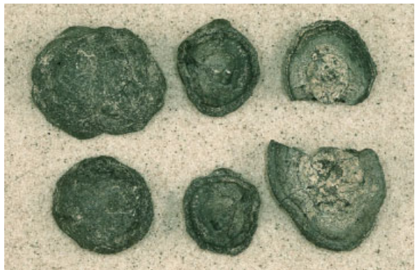
M42 Manganese nodules , built up of concentric layers of manganese and iron oxides. Brought up from the bottom of the ocean south-east of the Hawaiian Islands by Scripps Institute of Oceanography. The specimens given to the School of Mining and Metallurgy in Filipstad, Sweden by Professor Gustaf Arrhenius.
