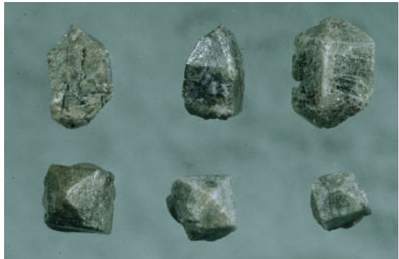
M30 Zircon \text{ZrSiO}_4 , tetragonal crystals. From Brevik in Norway. The prismatic form is visible in combination with the pyramid.
