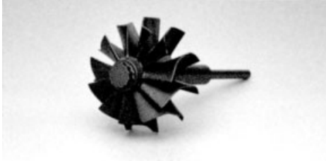
Figure 44.4 A silicon nitride component produced to its end shape. Nitride powder is encapsulated in glass and “hipped” (HIP
