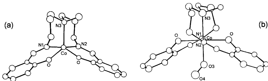
Figure 12 X-Ray structures of: (a) [Co(MeHsaldpt)] . Bond lengths: Co-O = 1.97 Å; Co-N3 = 2.15 Å; Co-N1 \approx Co-N2 = 2.04 Å; (b) [Co(MeHsaldpt)O_2] . Bond lengths: Co-O_{(Schiff\ base)} = 1.92 Å; Co-O3 = 1.88 Å; Co-N1 = 1.90 Å; Co-N2 = 2.00 Å; Co-N3 = 2.09 Å; Co-O3-O4 = 137.4^\circ
