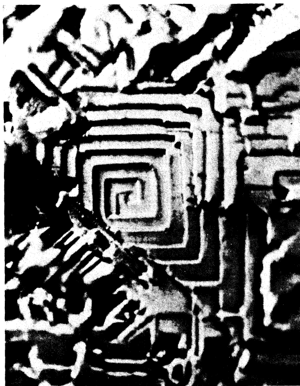
Fig. 5.50 Spiral growth of Cu from a 0.5 M \text{CuSO}_4 + 0.5 \text{ M H}_2\text{SO}_4 electrolyte, 25°C, current density 15 \text{ mA} \cdot \text{cm}^{-2} , magnification 1250 \times . (From H. Seiter, H. Fischer, and L. Albert, Electrochim. Acta , 2, 97, 1960)
