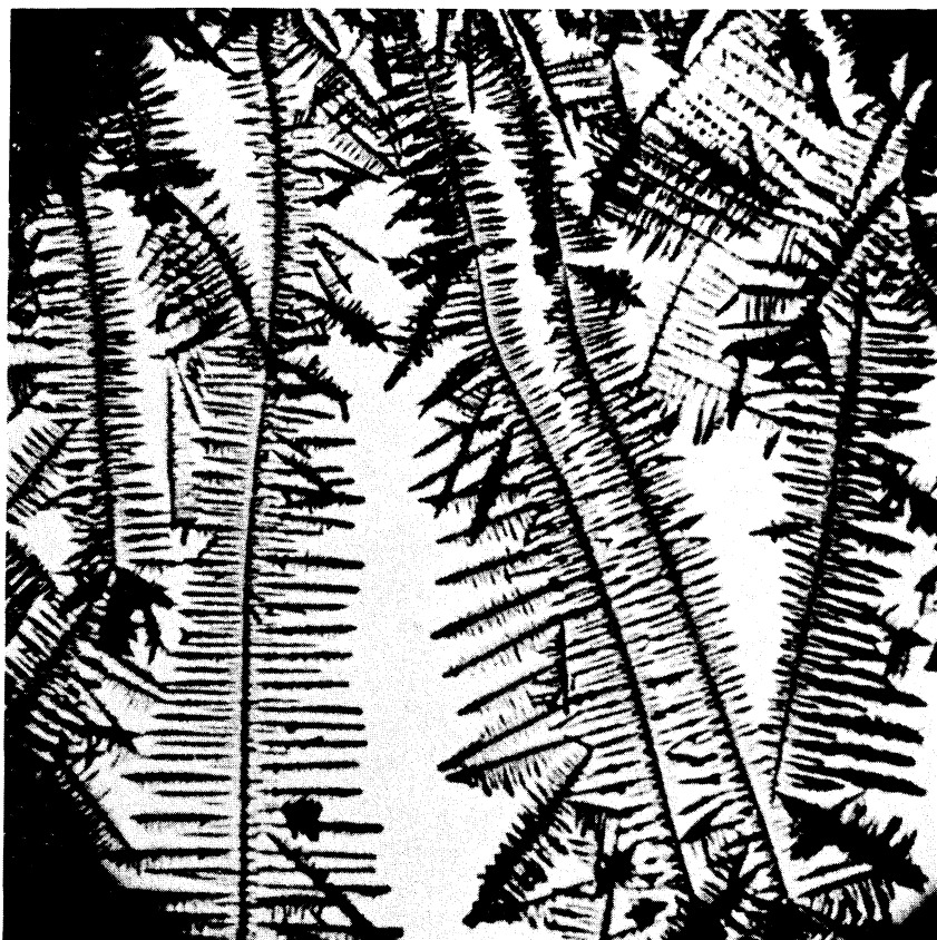
Fig. 5.52 \text{PbO}_2 dendrite growth at a lead electrode. Current density 0.3 \text{ mA} \cdot \text{cm}^{-2} . (From G. Wranglén, Electrochim. Acta , 2, 130, 1960)
