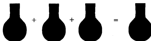
Figure 9.7 Dalton's Laws of Partial Pressure states that in a mixture of gases each gas exerts a pressure independent of the other gases. The total pressure is the sum of the partial pressures
