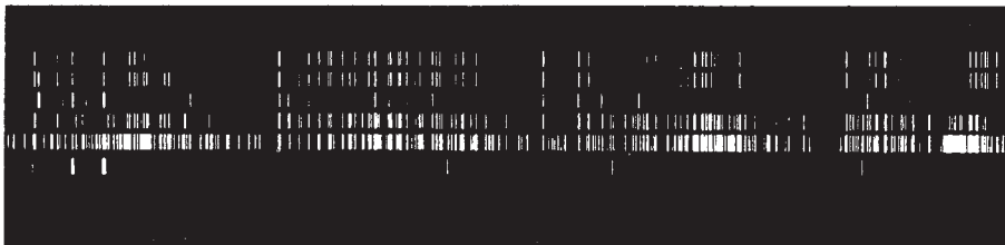
The lowest spectrum is that of copper and the one immediately above it is iron. The remainder are the spectra of ore samples. [The spectra are printed as 'positives' so that the emission lines appear white on a dark background.]
