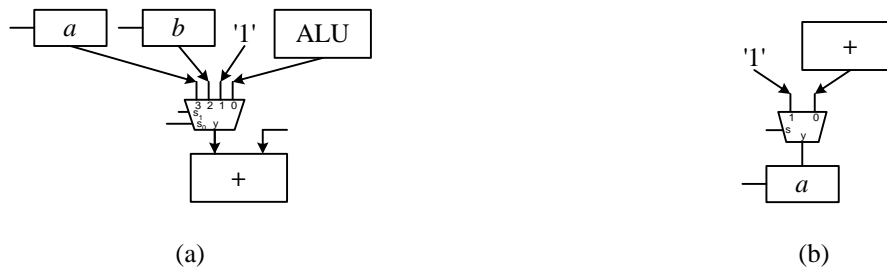
Figure 15. Examples of multiple sources using multiplexers.
