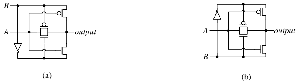
Figure 15. CMOS circuit using only six transistors for: (a) XOR gate; (b) XNOR gate.
