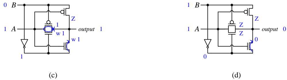
Figure 16. Analysis of the CMOS XOR gate circuit. (a) shows the analysis for the inputs A=0 and B=0 . All the transistor outputs are annotated with the resulting output value. The letter “w” is used to signify that it is a weak value. (b) to (d) show the analysis for the remaining input combinations.
