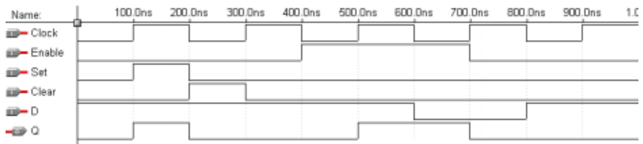
Figure 27. Simulation trace for the positive-edge-triggered D flip-flop with active high enable and asynchronous set and clear.
