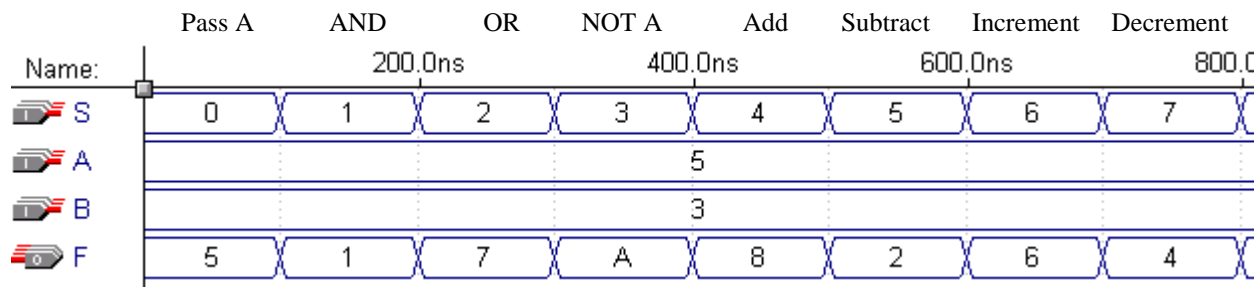
Figure 14. Waveform generated for the two input operands 5 and 3 for all of the eight operations.
