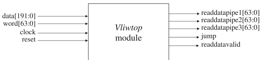
Figure 3.16 Diagram showing interface signals for vliwtop module.
