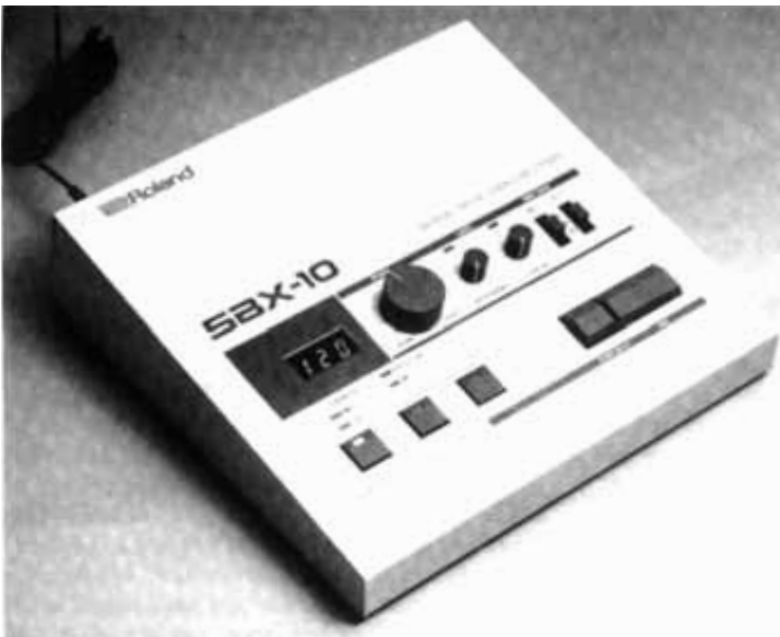
Figure 20.10 A MIDI-compatible synchronizer – the Roland SBX-10.
