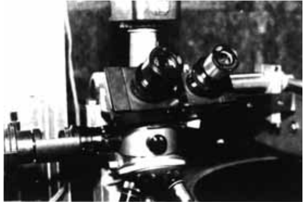
Figure 9.2 Stereo binoculars used to check the cut groove – a TV monitor is also used for checking.
