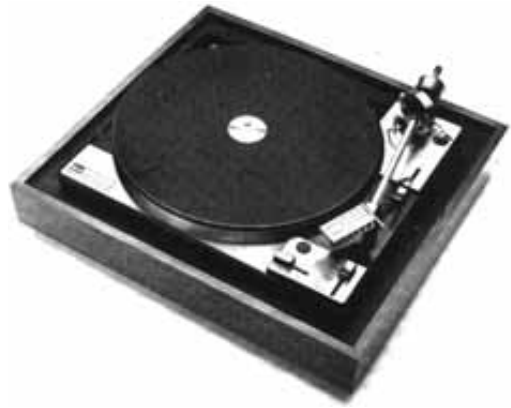
Figure 9.4 A typical older type of playing deck unit.
