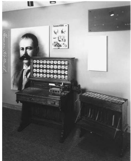
A portrait of Herman Hollerith next to one of his punch card tabulator machines. Such machines made it possible to complete the 1890 U.S. census in a fraction of the time needed by earlier methods. (Photo courtesy Computer Museum History Center)
