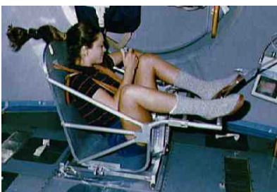
g / Astronaut Tamara Jernigan measures her mass aboard the Space Shuttle. She is strapped into a chair attached to a spring, like the mass in figure f. (NASA)
