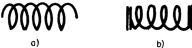
FIGURE 8.12 a) Spring design not recommended for automatic handling; b) Design of a spring more suitable for automatic handling.
