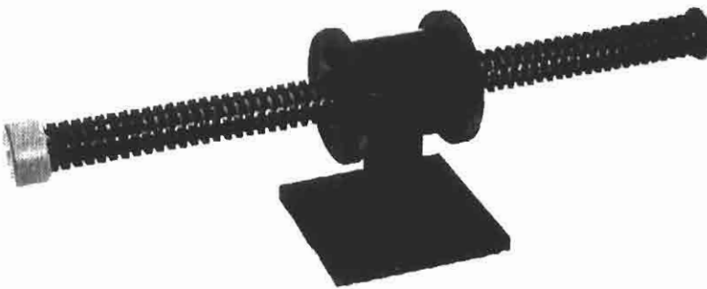
FIGURE 9.20a) General view of the manipulator having two degrees of freedom, which is shown schematically in Figure 9.20. Built in the Mechanical Engineering Department of Ben-Gurion University. This device was patented by RoBomatex Company in Israel.
