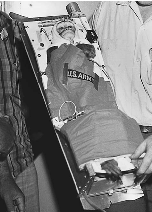
Launch support personnel prepare to place Able, a female rhesus monkey, into the special capsule within the nose cone of the U.S. Army's Jupiter AM-18 rocket, as part of preflight testing at Cape Canaveral. As shown in the photograph (taken on May 18, 1959), the American-bred monkey is restrained on a special launch couch and extensively instrumented with implanted medical electrodes. (NASA)
