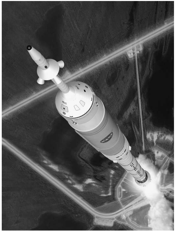
This is an artist’s rendering of NASA’s new crew launch vehicle, called Ares I, taking off from the Kennedy Space Center in Florida, circa 2015. The two-stage rocket is shown topped by the crew exploration vehicle, its service module, and a launch abort system. (NASA/MSFC)
