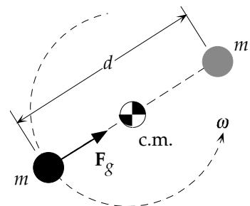
The absolute acceleration of  $m$  is normal to its circular path around c.m.,
