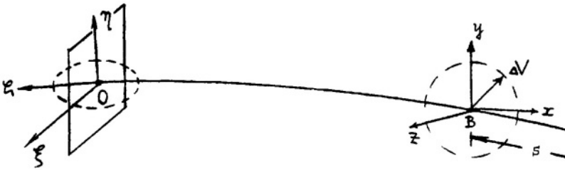
Figure 10.2. Heliocentric segment of a nominal SC trajectory passing through the center O of a planet
