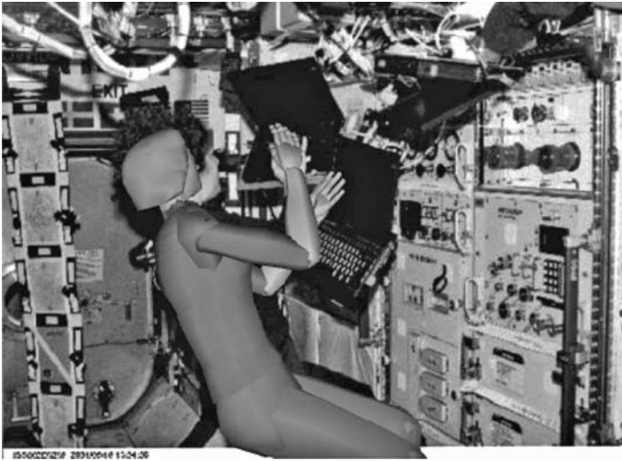
FIGURE 13.2 Virtual mannequin (JACK®) analysis (Courtesy of NASA and Alcatel Alexia Space, Italy).
