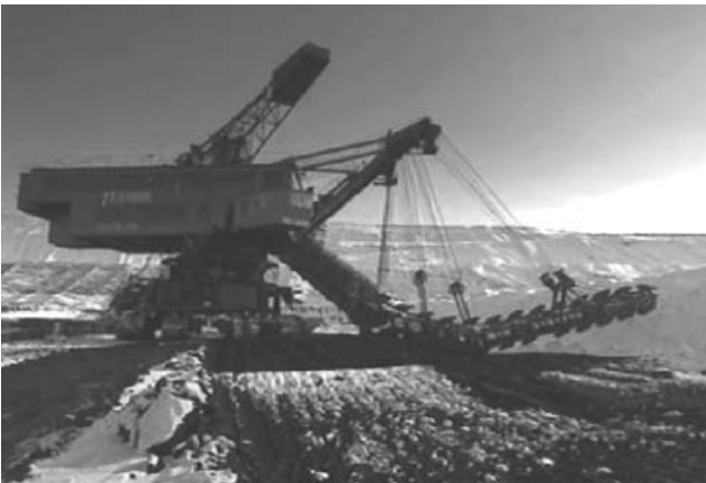
FIGURE 32.3 Excavator in bucket-ladder configuration—terrestrial application.
