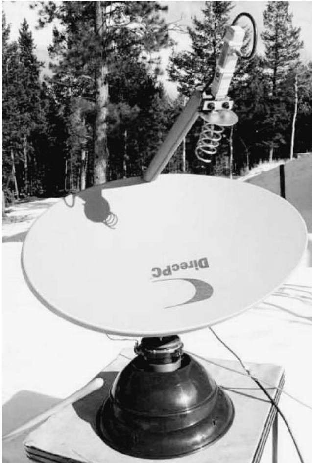
Figure 4.37 Helical fed reflector antenna (Reproduced by permission of © Dr. Robert Suding/ultimatecharger.com)
