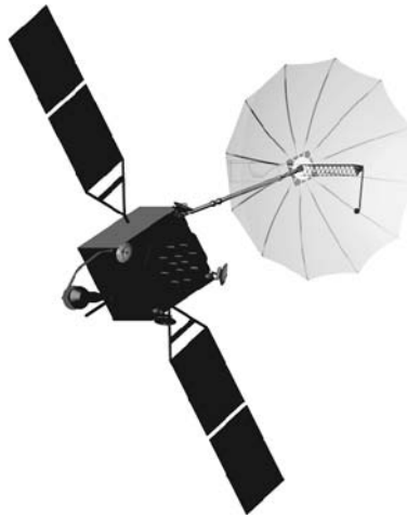
Figure 12.6 Block-IIF GPS satellites (Reproduced by permission of © Aerospace Corporation)
