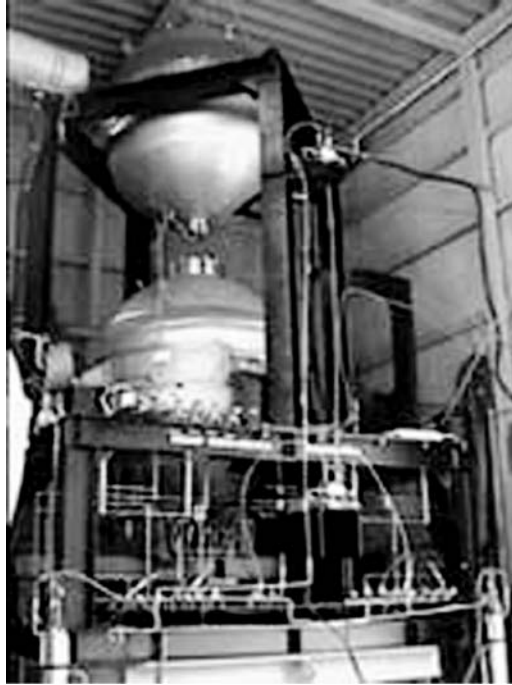
Figure 4.6 Bipropellant propulsion system used on board ETS-VIII Satellite (Provided by the Japan Aerospace Exploration Agency (JAXA))
