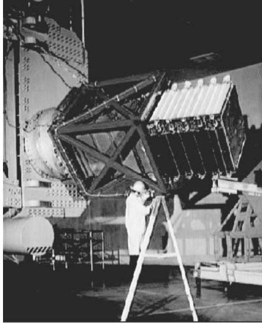
Figure 4.12 Heat pipe thermal control system onboard the third space shuttle mission (STS-3) (Courtesy: NASA)
