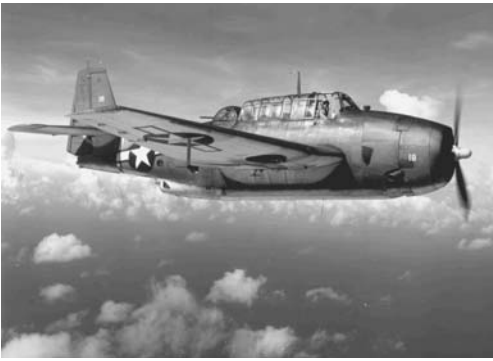
The TBM was the largest single-engine aircraft used in World War II. It was designed to carry three crew: pilot, gunner, radioman. (National Archives)
