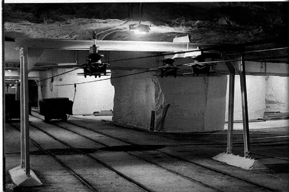
15. No. 10 District haulageway in 1938, showing the newly installed rope-haulage system under test. Note the special quick-release clip connecting the haulage chain to the rope.
