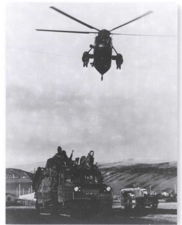
A Fleet Air Arm Sea King helicopter flies over a Bv 202E of 45 Commando as it drives out of Port San Carlos on 21 May 1982. The Sea King HC4 could carry 28 fully equipped men or an underslung load such as a light gun. In training Fleet Air Arm crews work closely with the Royal Marines in challenging and hazardous environments. (RM Museum, 7/20/18 (130))
