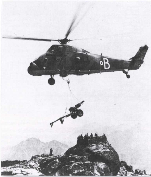
A Westland Wessex helicopter brings in a 105mm pack howitzer as an underslung load to a mountain position in the Radfan. The Italian-designed pack howitzer would give invaluable service both in the Radfan and the Indonesian Confrontation. Designed for mountain operations, it could be broken down into loads that could be carried by mules. (Author's collection)
