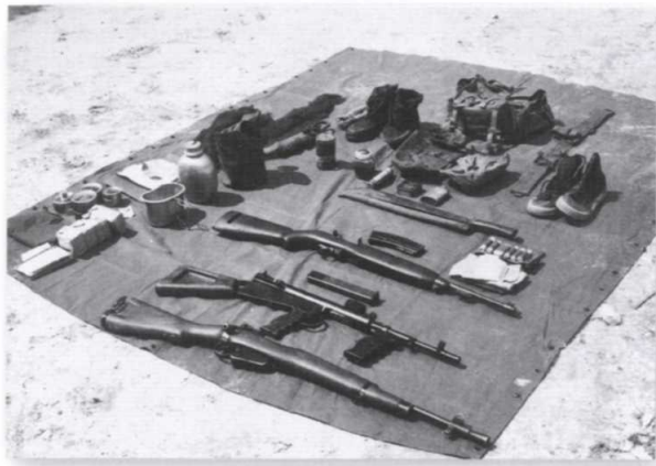
ABOVE LEFT The weapons and equipment carried by Royal Marines during the Emergency in Malaya in the 1950s, including 1944-pattern webbing, the excellent aluminium mug and machete. The commando would have had a choice of several weapons. Shown here are the American M1 carbine, Australian Owen submachine gun (SMG) and the No. 5 jungle carbine. While the 9mm Owen looked clumsy, it was very reliable. The elegant No. 5 had a 'wandering zero', which meant that the sight settings would go out of alignment, and it had a vicious recoil. (IWM MAL 300)
