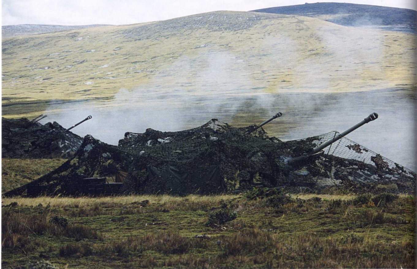
105mm light guns fire on East Falkland. The Commando gunners were invaluable in their ability to provide quick and accurate fire in support of the attacks against the defended features that blocked the western approaches to the island's capital Stanley. The guns could fire a 35 lb (15.8kg) shell a distance of 10 miles (16km). (Media Ops, Land Command)
