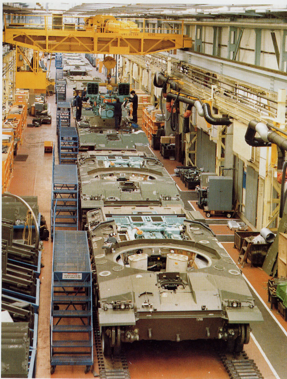
(Right) Following an initial MOD order placed in September 1979 for 243 MBTs at a cost of £300 million, production of Challenger was undertaken at the Royal Ordnance Factory at Barnbow in Leeds. Here, the 1,200bhp powerpack is being fitted on the hull assembly line. Barnbow has been one the most important tank factories in Britain, producing AFVs since the Second World War. In July 1986 Vickers Defence Systems purchased the factory following the privatization of Royal Ordnance Factories; and in 1998 VDS announced that Barnbow was to close.
