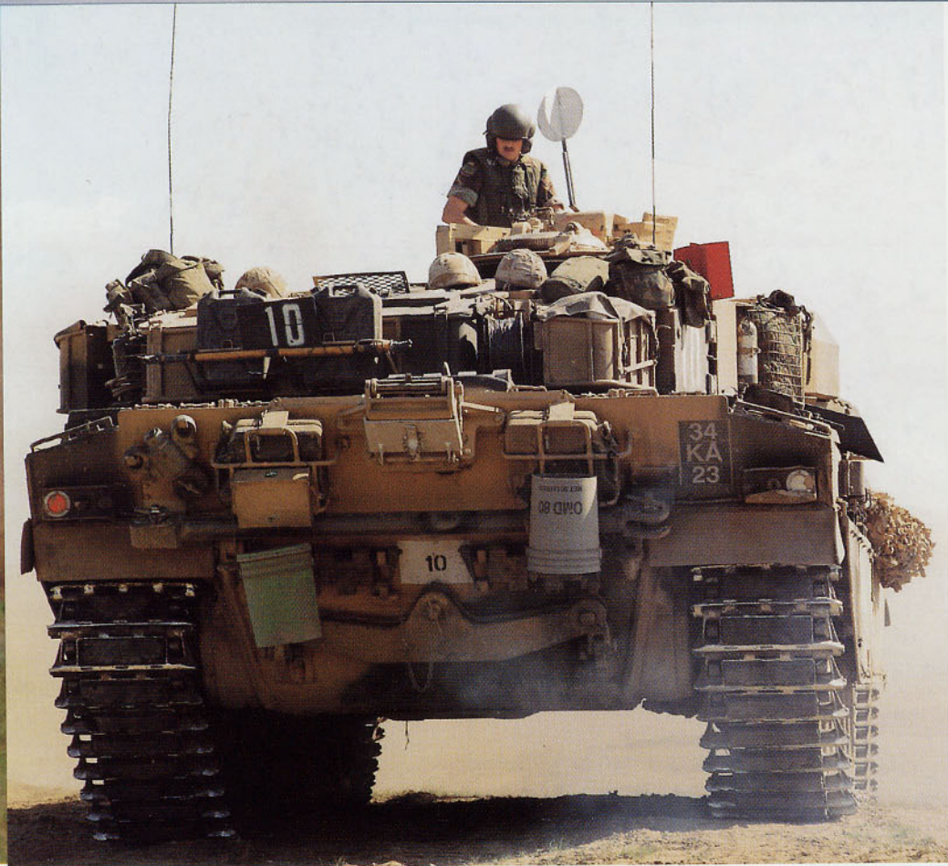
(Right) This photograph of a Challenger 1 Mk 2 of the BATUS 1st Armd.Sqn. shows to advantage the TOGS, and the white painted V on the turret roof, which is known as the 'forty-fives'. Visible through both the commander's and gunner's sights, the 'forty-fives' are aligned with either the right or left front trackguard, as ordained by range controllers to determine safe arcs of fire when using live ammunition. Note the Thermal Imager Sensor Head (TISH) inside the open door of the TOGS barbette.
