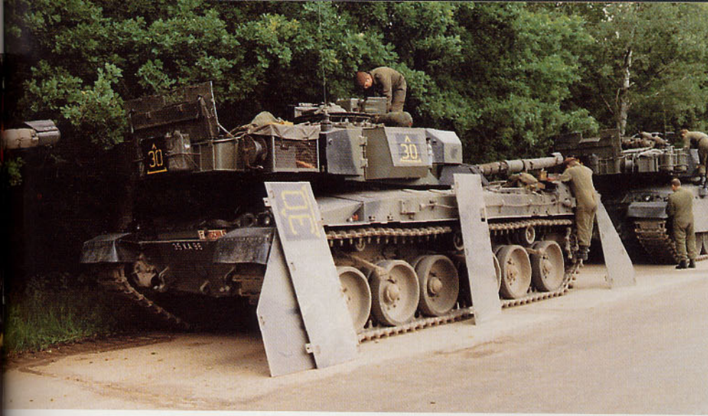
(Left) The complexity of modern MBTs demands regular maintenance procedures; here, hidden from aerial view, Challenger crews of The King's Royal Hussars carry out routine maintenance prior to an exercise, from lubrication of the suspension units to cleaning the 120mm main armament. (Simon Dunstan)
