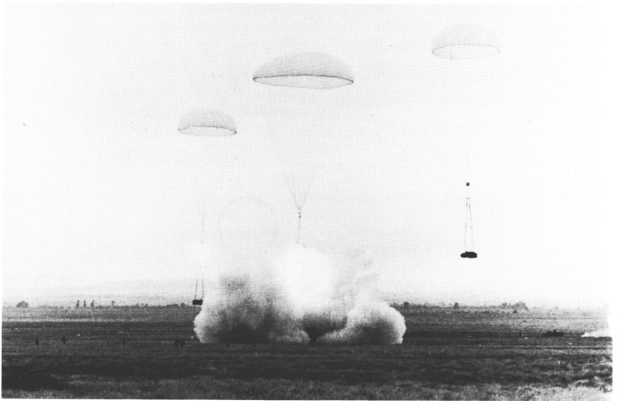
The Soviets have pioneered the use of heavy platforms for airborne landings; these appear to be BMD platforms. Posts protrude beneath the platforms, triggering a retro-rocket to soften the impact of the main structure.
