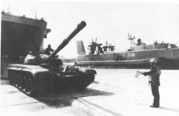
The mammoth AIST hovercraft are currently being adopted by the Soviet Navy in larger numbers; they are capable of carrying tanks, as evident in this view of a disembarking T-74. The Soviet Naval Infantry pioneered the use of hovercraft in amphibious landings. (Sovfoto)
