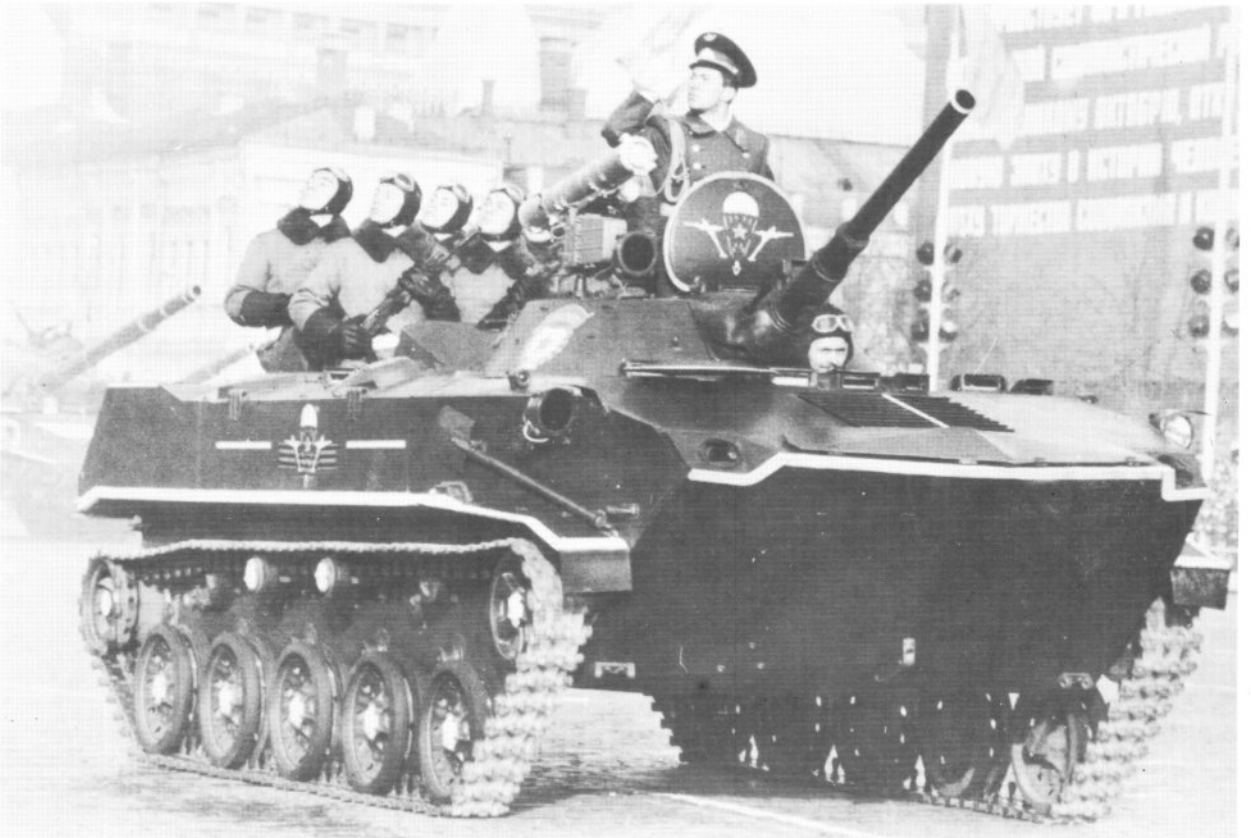
(Above) The re-engineered BMD-1M's most recognisable features are the new 'sunburst' pattern wheels replacing the earlier 'spoked' wheels; and the new grills in the upper hull front plate to improve ventilation. (Sovfoto)
