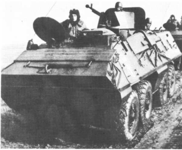
Though much more lightly mechanised than comparable Soviet formations, the Polish 6 PDPD has a modest number of OT-64 SKOT armoured personnel carriers.
