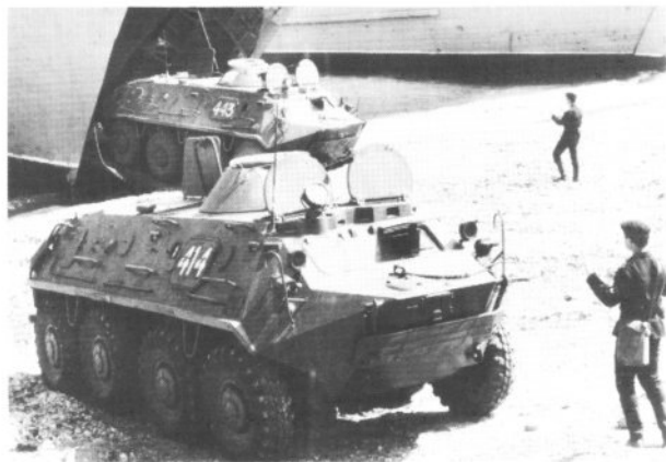
The principal armoured vehicle of the Naval Infantry is the BTR-60PB; these have only limited amphibious capability, and are as often as not landed on or very close to the beach from their Polnocny LSTs. (Sovfoto)
