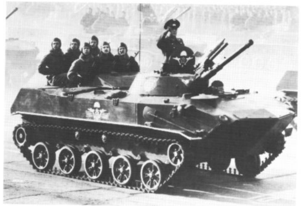
The BMD-1 Model 1973 has been the standard production version of this unique vehicle. It has the improved circular CBR air vent as compared with the square vent of the earlier Model 1970. This parading BMD is marked with the Guards insignia on the turret, and on the hull side with the badge shown as our Plate L2. (Sovfoto)
