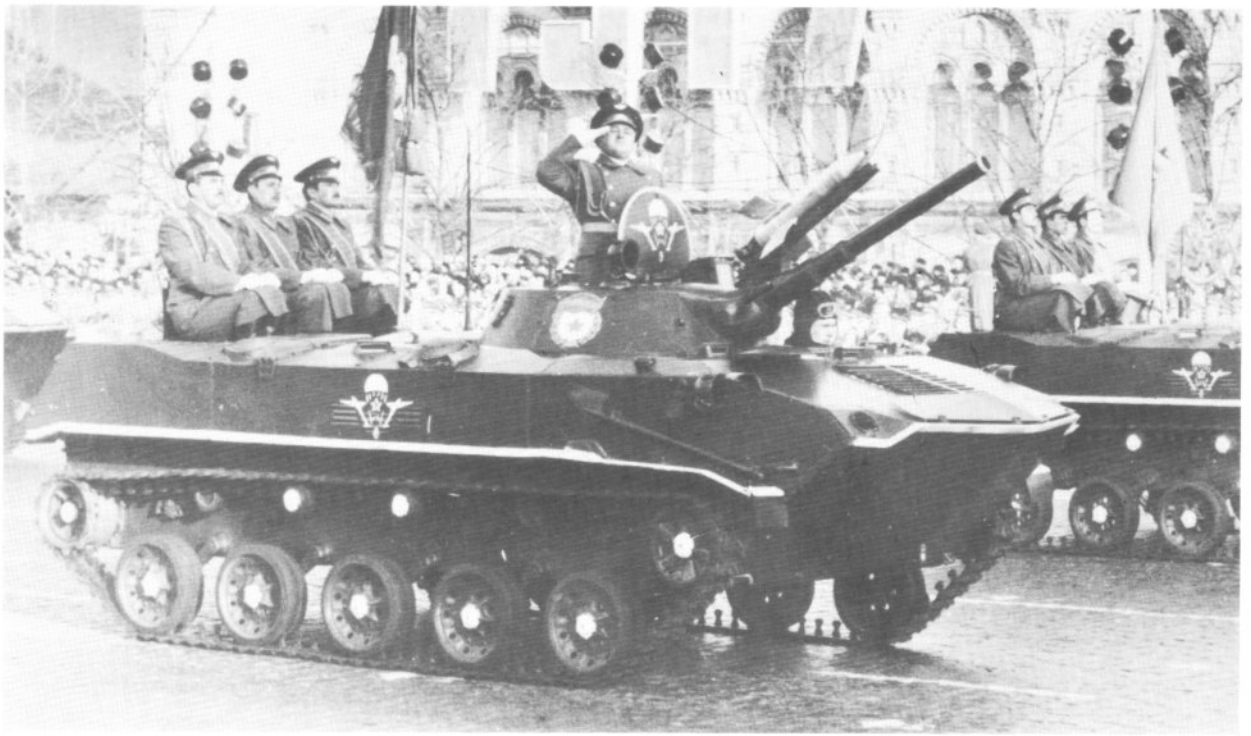
(Above) The re-engineered BMD-1M's most recognisable features are the new 'sunburst' pattern wheels replacing the earlier 'spoked' wheels; and the new grills in the upper hull front plate to improve ventilation. (Sovfoto)
