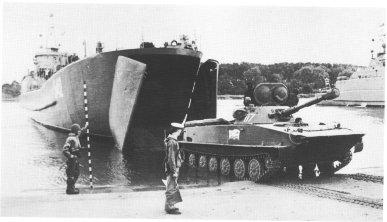
The elderly PT-76's amphibious capability makes it the principal tank of the Naval Infantry forces. The Polnocny class LST, seen here, represents the bulk of the Soviet landing ship fleet; it is in fact of Polish construction, being built at Gdansk—the Polish designation is ODS. (Sovfoto)
