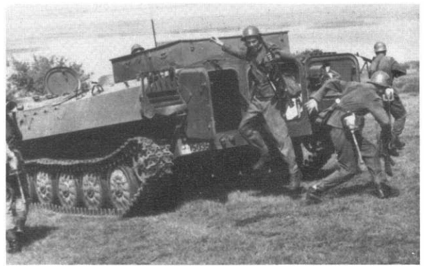
A Bulgarian motorised rifles squad dismounts from an MT-LB armoured personnel carrier: while not primarily intended as an APC, it is employed by some WP forces in this rôle as a low-cost alternative.
