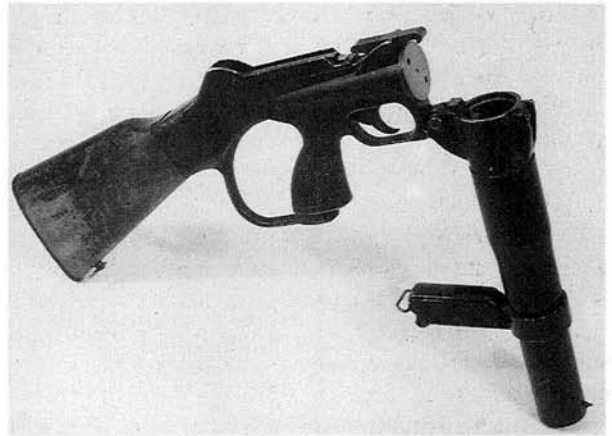
The Webley-Schermuly riot gun is one of a number of weapons used by the Security Forces in public order situations to fire plastic bullets. (AIS HQ NI)
