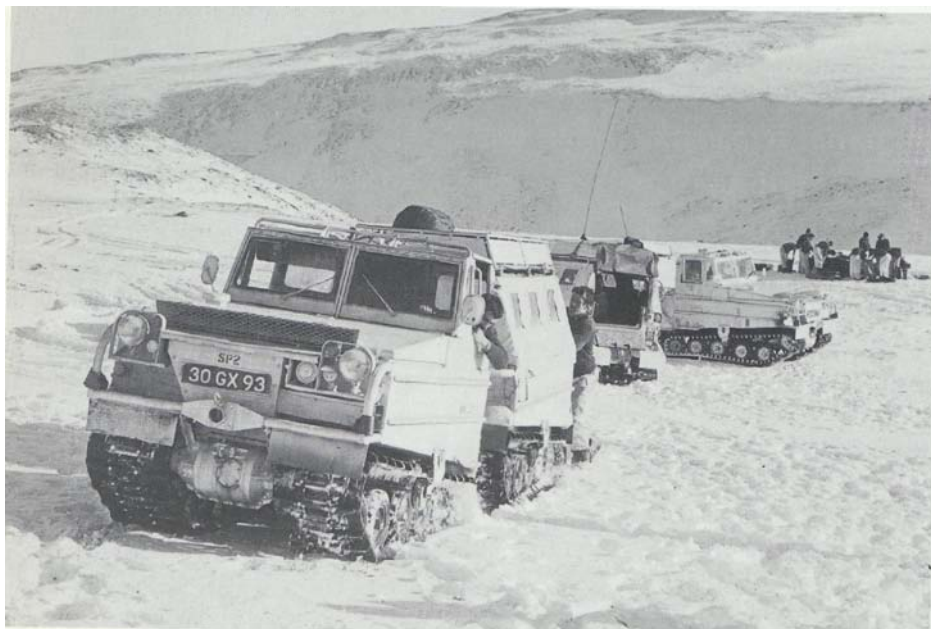
Swedish built Bandvagn Bv202 over-snow vehicles in Norway. The Royal Marines took these to the Falklands in 1982 where they proved effective in negotiating the soft peat of the islands. They have now been replaced in the UK by the larger and more powerful Haaglund Bv206. (W. Fowler)
