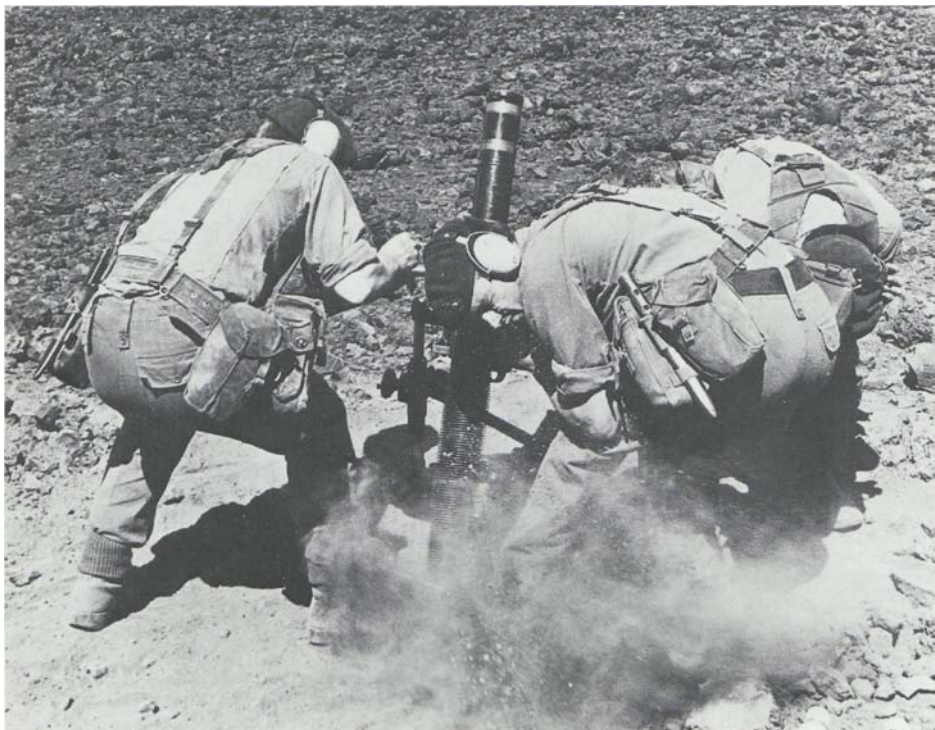
Royal Marines fire the 81 mm L16 mortar during training on Ascension Island in 1982, prior to Operation Corporate on the Falkland Islands. The L16 can fire 15 rounds per minute for indefinite periods, and also be broken down into three loads which can be man packed. (W. Fowler)
