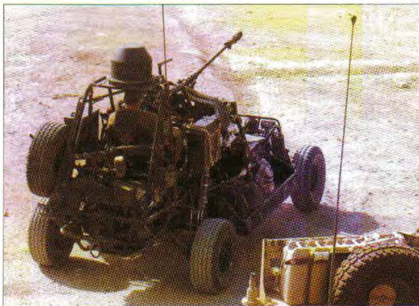
Part of the SEALs' considerable arsenal is the Desert Patrol Vehicle (DPV). It is basically an off-road racing vehicle, intended for use anywhere a four-wheel-drive vehicle can go, but with additional speed and maneuverability. It can carry a variety of weapons.
