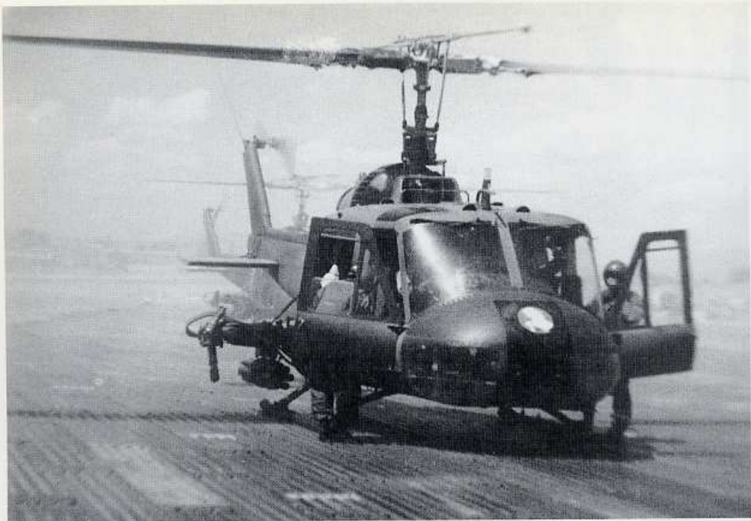
A UH-1C Huey gunship flown by Thai volunteers touches down at Pakse airbase, 1972. It is armed with 2.75 in. rockets and an XM-21 7.62mm flexgun system. A white horse—the radio call sign for UH-1C support in Laos—is painted on the nose of the helicopter.
