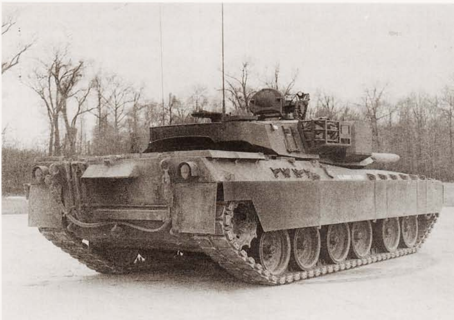
A rear view of the General Motors XM1. This vehicle had far less prominent exhaust venting at the rear than the Chrysler XM1 since it used the AVCR-1360 diesel engine. (US Army)
