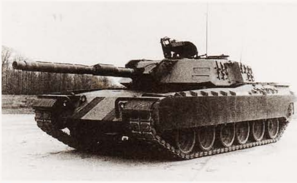
The XM1 development programme was a competitive effort between General Motors and Chrysler. Seen here is the General Motors validation phase tank. (US Army)
