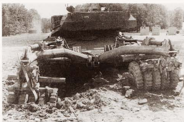
The BCS also includes a mine roller, patterned after Soviet systems. This photo was taken during tests at
