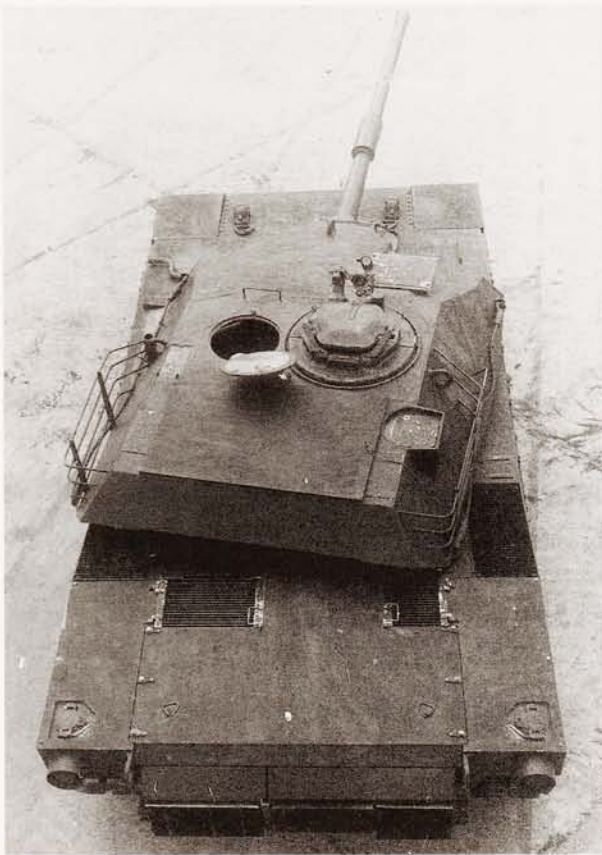
An overhead view of the Chrysler XM1 validation phase tank. There were many changes to the turret
