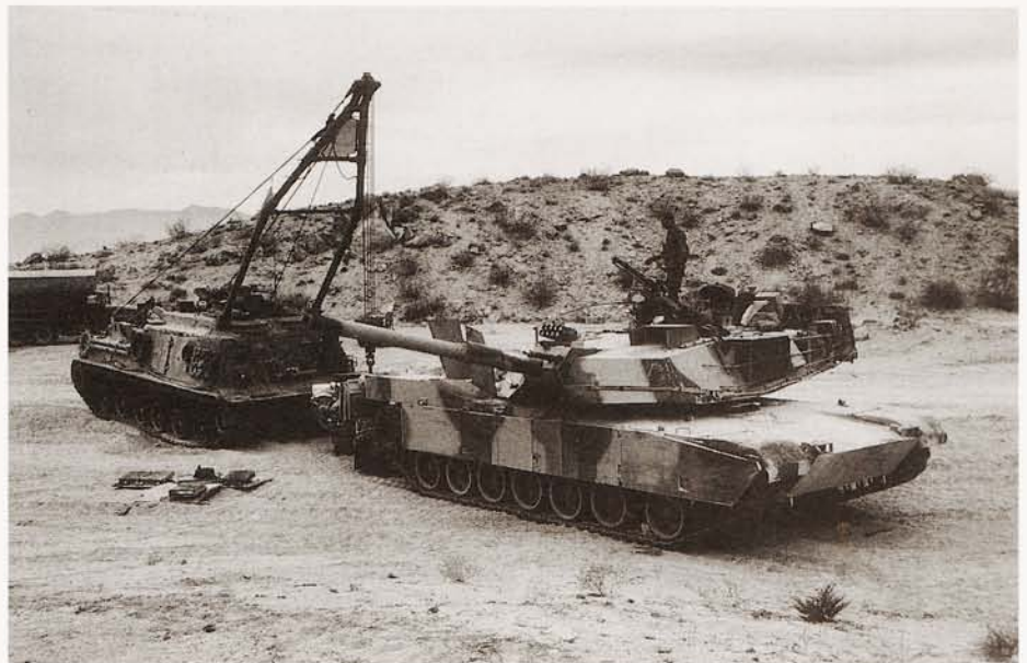
An IPMI undergoes repairs by an M88 recovery vehicle at the National Training Center at Ft Irwin, California. Most US tankers feel that the realistic war-games at NTC were the prime reason for the outstanding performance by US armour units during Desert Storm. (Author)
