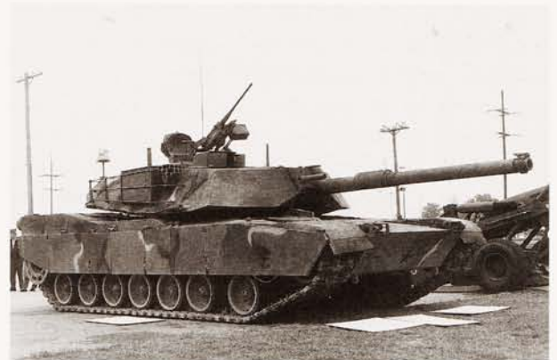
One of the initial low-rate-initial-production M1 Abrams tanks at Aberdeen Proving Ground shortly after their introduction into service. The XM1 FSED tanks can be distinguished by a more complicated ammunition feed on the
