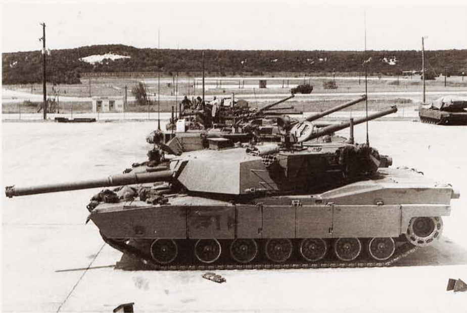
The 2nd Armored Division was the first unit to re-equip with the M1 in 1982-83. One modification developed at Ft Hood was to cut back the rear skirt to prevent mud from building up in the drive sprocket. This was later adopted at the factory. The markings on the hull side identify this vehicle as belonging to the 'Hounds of Hell' 3-67 Armor. (Author)
