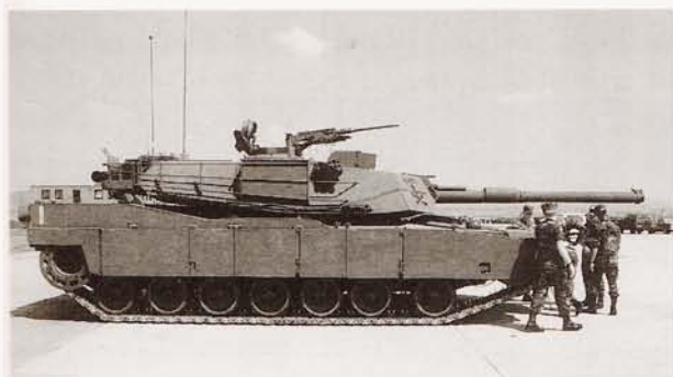
Another example of a modernised M1 Abrams with the rear turret basket, this time Ballbuster, the command tank of B Troop, 1-11 ACR at Fulda, Germany in 1988. The spacing between the front tow cable attachment and the turret armour joint on the right turret side is
