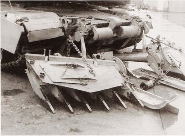
The most common element of the Battalion Counter-mine Set (BCS) is the mine plough. This system is
