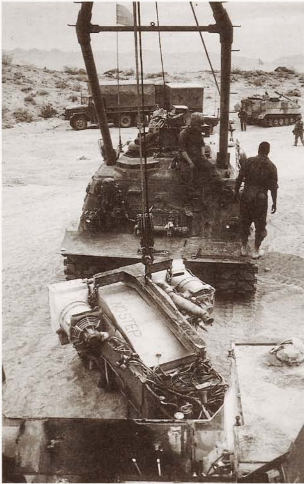
An AGT-1500 gas turbine powerpack is pulled from an IPM1 Abrams at NTC by an M88 recovery vehicle. Although the turbine has
