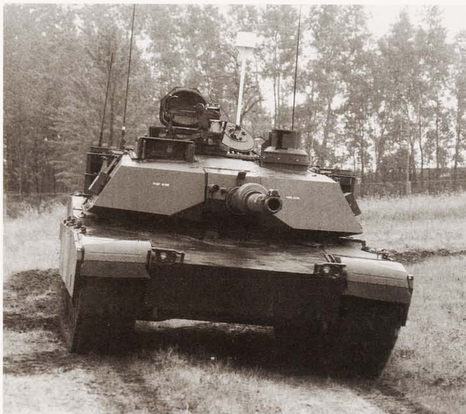
A frontal view of the M1A2 Abrams during trials. In this view, two of the key external changes: the ICWS cupola and CITV sensor can be seen. (GDLS)
