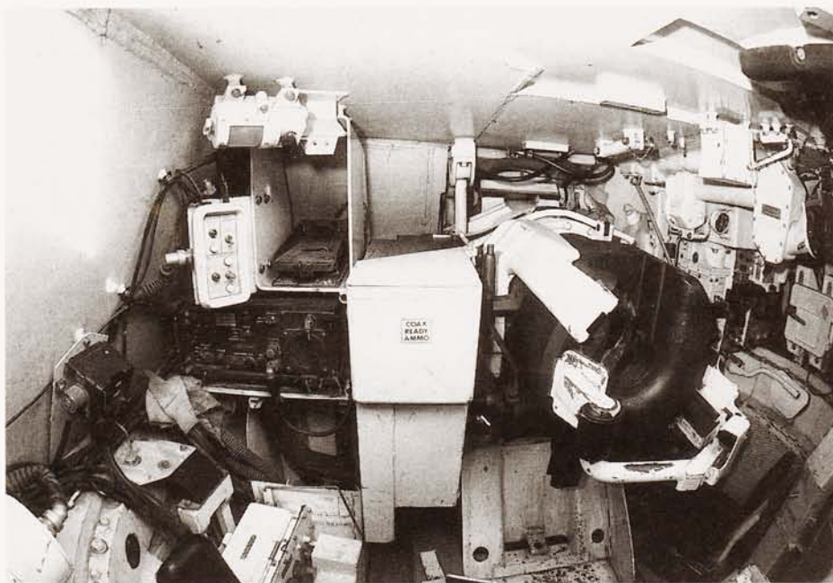
An interior view of the M1 looking forward in the loader's station showing the vehicle radio to the lower left and the gun breech to the right. (Author)
