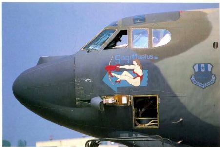
Above The waveguide antennae are clearly visible beneath the female archer on the nose of 58-0252, otherwise known as Sagittarius II
