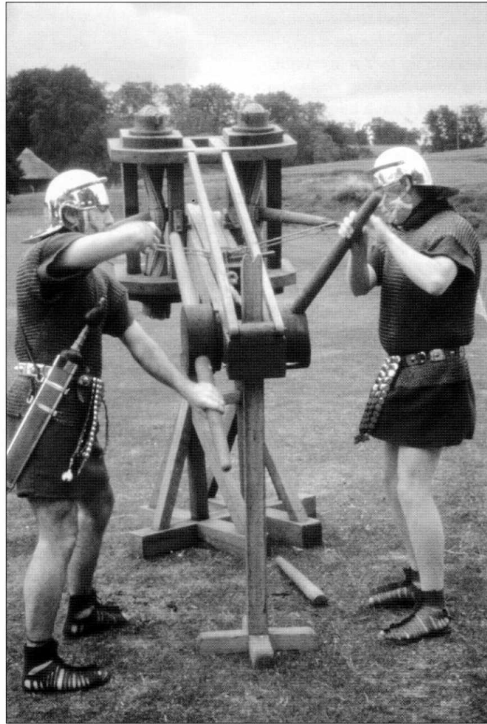
The ballista belonging to the Ermine Street Guard re-enactment group is the optimum size to launch stones weighing around 4 Roman pounds (1.3kg). Even such a lightweight catapult requires considerable space to operate efficiently. (© Ermine Street Guard)
