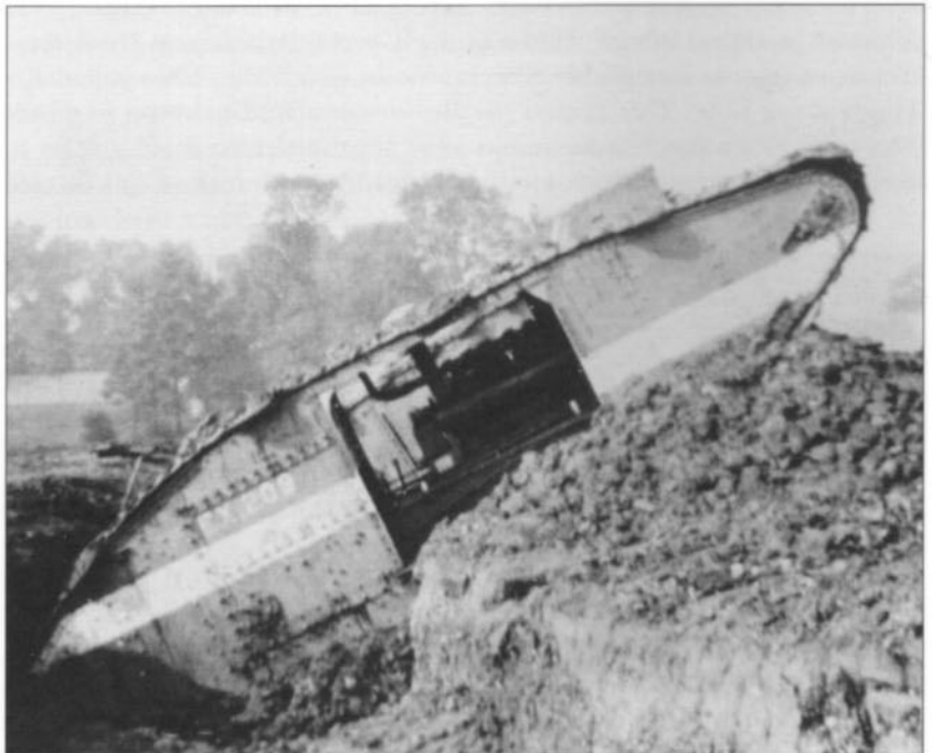
Experimental machine 209, one of the Oldbury Trials tanks, crossing a trench at Dollis Hill. The broad coloured stripe served to identify competing machines. The five Mark II tanks all ran without sponsons and many other detail fittings were not attached.
