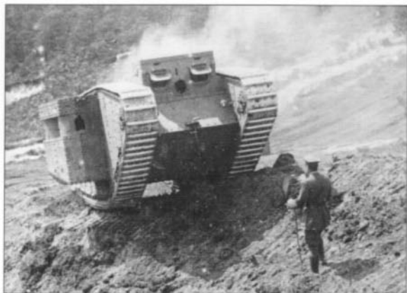
BELOW An excellent view of a Mark III Female with the smaller Lewis gun sponson. The escape hatches below the sponson are wide open and the two rotating shields for the machine guns have been turned to face inwards. Notice also the clevises, or hooks, at each end of the sponson for lifting it off.
