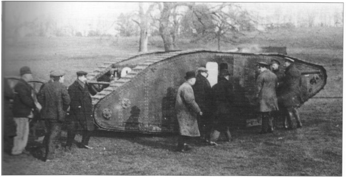
Tritton, Wilson and Stern are among the group gathered around Mother's starboard sponson. Notice how the door swings outwards but against the hull. The small, oval door at the rear is also open and can just be seen over the tracks.
