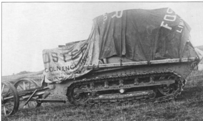
Draped with tarpaulin covers to disguise its warlike purpose, the Lincoln Machine is shown during trials. This photo was taken after the tracks had been modified, but they still proved unsuitable for the work they would have to do.
