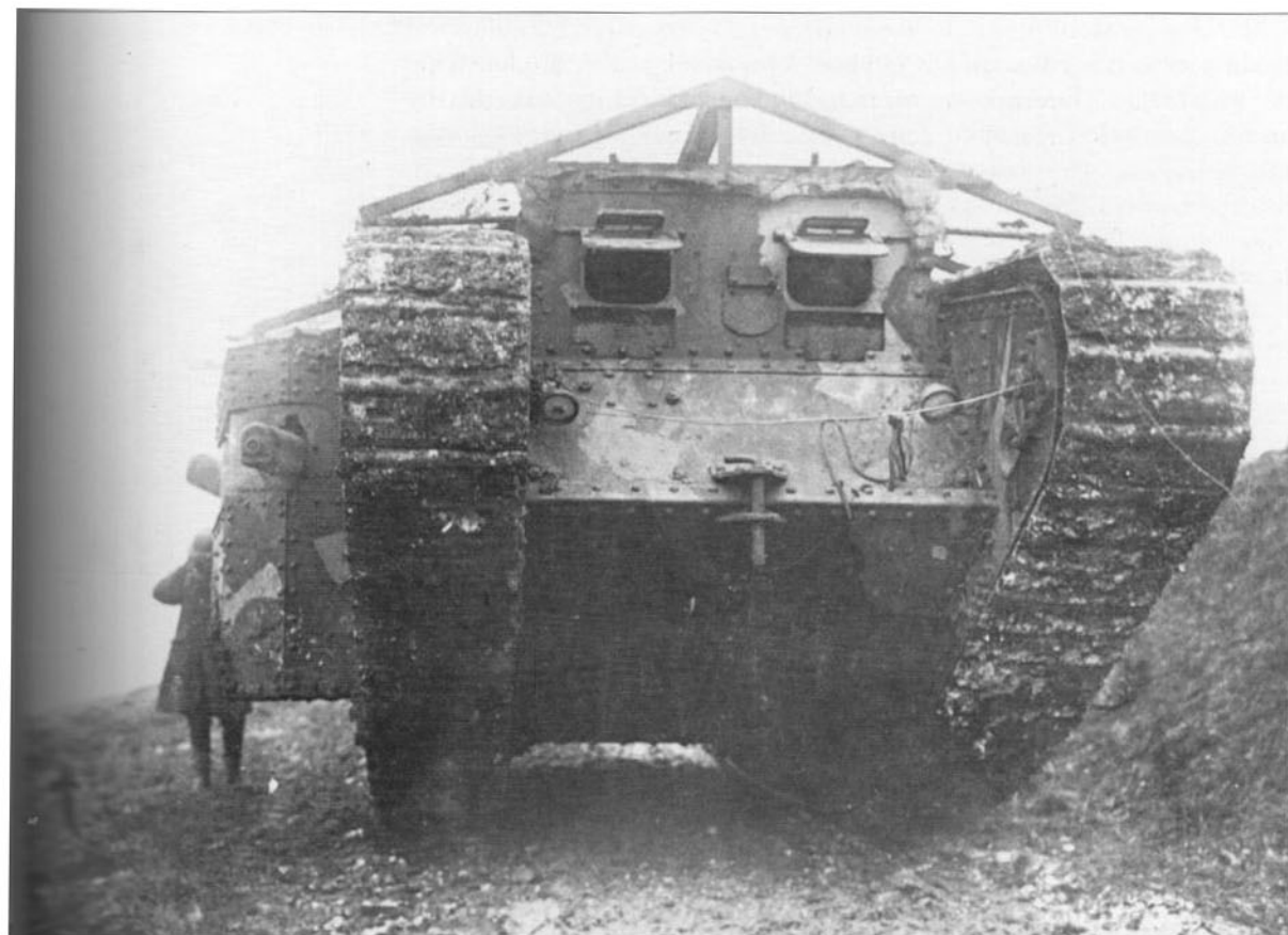
Close-up frontal view of a Female Mark I, probably of A Company during the November 1916 actions. This company also employed the grenade-proof roof, but this one seems to have an extension over the top of the sponson, which would make sense.
