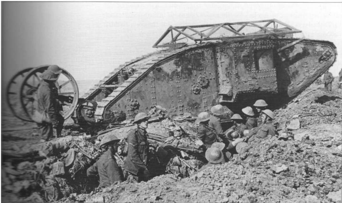
Another classic photograph; C15 moving up for the attack on Thiepval on 26 September 1916. Mud is thickly plastered at the front and seems to have obliterated much of the camouflage. The tank is running with its tail clear of the ground, the gun on full elevation and doors shut.
