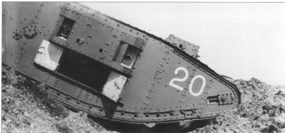
BELOW An excellent view of a Mark III Female with the smaller Lewis gun sponson. The escape hatches below the sponson are wide open and the two rotating shields for the machine guns have been turned to face inwards. Notice also the clevises, or hooks, at each end of the sponson for lifting it off.
