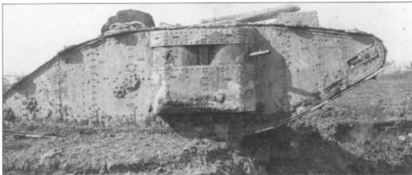
A Mark II Female, The Perfect Lady , at Arras. The camouflaged sponson must have come from a Mark I but it now carries a pair of Lewis guns. It seems that the crew have painted artificial vision slits on the hull and sponson sides. German soldiers were ordered to aim specifically at vision ports.
