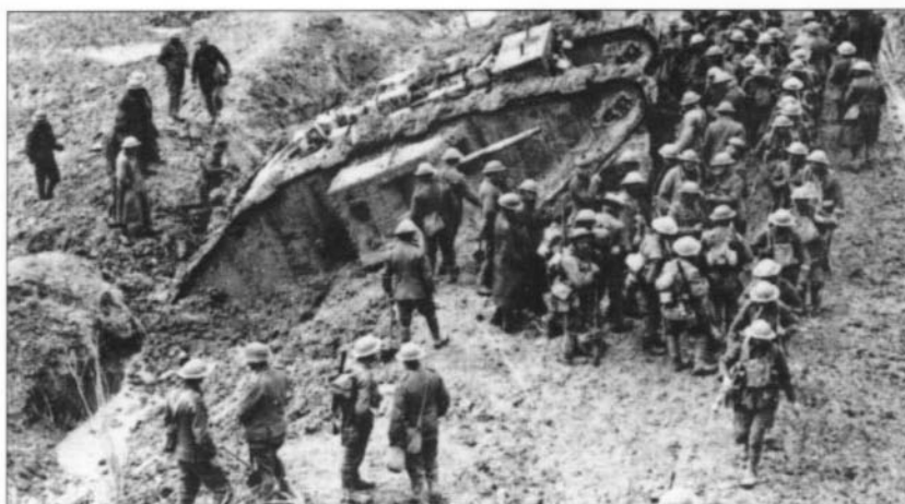
The only known view of a Mark I at Arras, 2nd Lieutenant Tarbet's C6 (No. 752) ditched close to the Blangy Road. Shorn of its tail and fitted with track extension plates it can only be identified by the shape of the track adjustment recess which is more rounded than on the Mark II.
