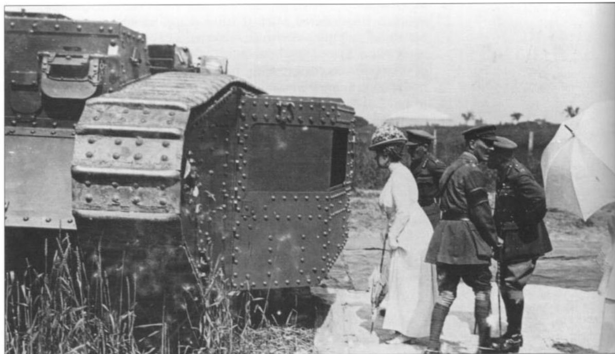
Queen Mary gazes into the blanked-off sponson of a Mark II supply tank. This is a good point to examine the rivet pattern along the top of the cab, which is a distinguishing feature of Mark II and III machines. This inspection took place at Neuve Eglise in the summer of 1917.
