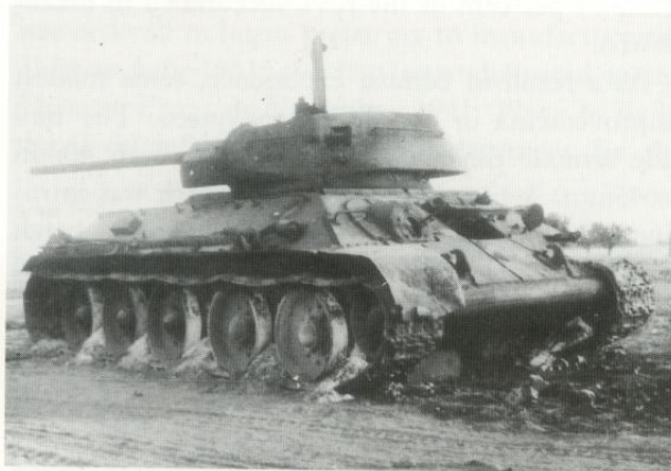
The T-34 Model 1942 was a simplified version of the Model 1941, introducing a new pattern of tracks, new driver's hatch and many other small features. This is a T-34 Model 1942 knocked
