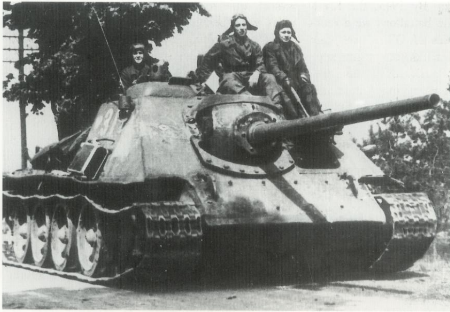
The 13th Self-propelled Artillery Regiment of the Polish LWP took part in the Berlin campaign in April-May 1945. Notice that the vehicle has lost its front roadwheel, presumably to a land-mine.
