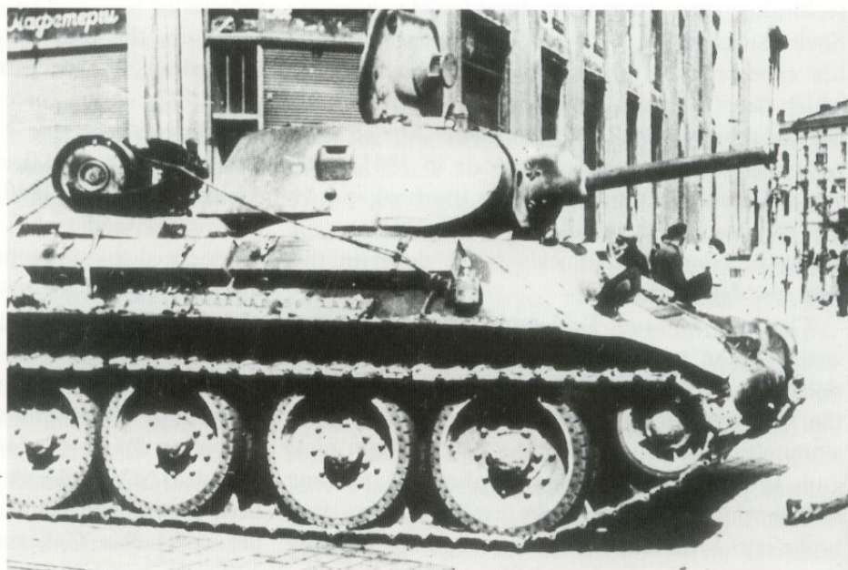
A T-34 Model 1940 of Vlasov's 4th Mechanised Corps, abandoned on the streets of Lvov in western Ukraine in June 1941. Strapped to the back engine deck is a spare transmission, a reminder of the teething problems suffered by the new machines. (US National Archives)
