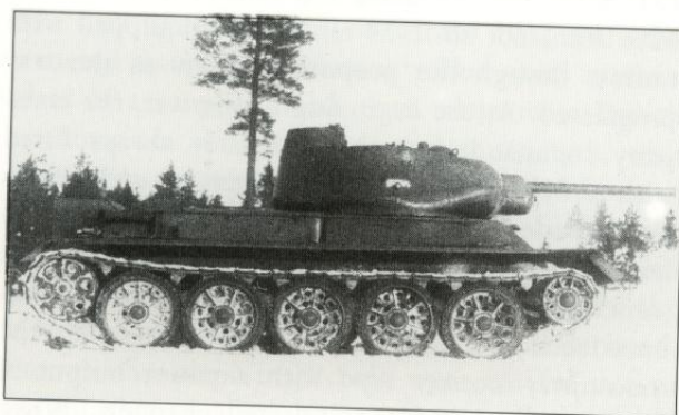
A second attempt to replace the T-34 was undertaken in 1942, under the designation T-43. Although closely resembling the T-34, it used torsion bar suspension,
