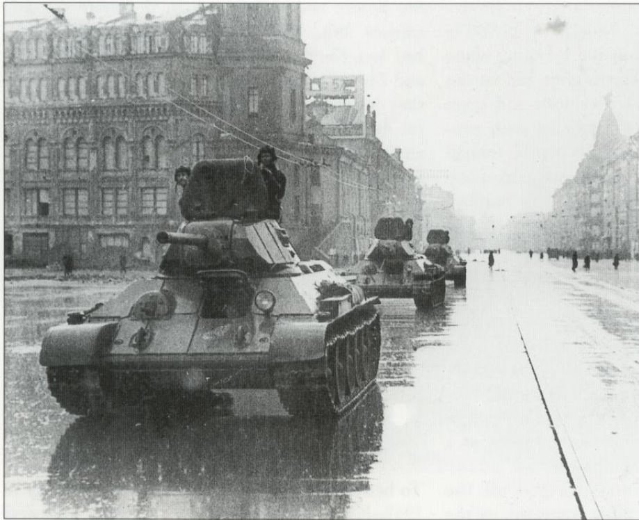
The STZ T-34s had many small differences from those at other factories, including the use of an interlocked glacis plate. These T-34 Model 41/42 tanks were rebuilt by Zavod No 27 in Leningrad with additional armour plate to better protect them against newer German anti-tank guns. Surprisingly, these were still in service at Leningrad in June 1944. (Sovfoto)
