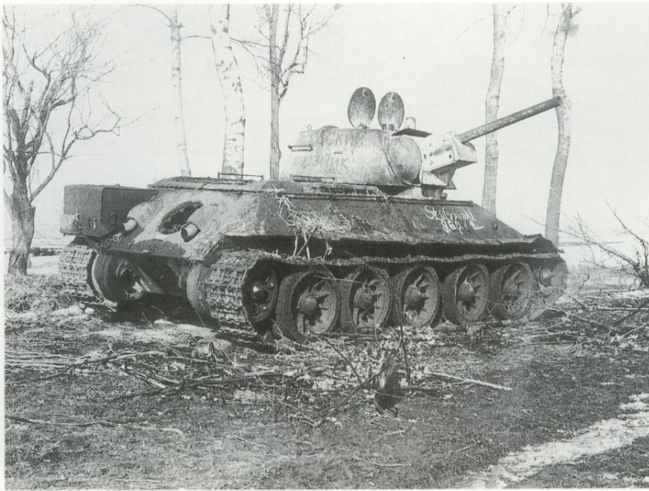
In the autumn of 1942, T-34s began to be fitted with external 40-litre fuel containers on the hull rear. This particular T-34 Model 1943, named 'Moskovskiy Khokolznik', appears to have had its right side container knocked off in combat. (National Archives)
