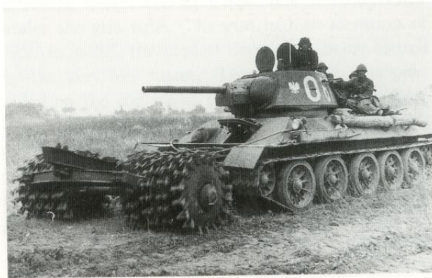
The PT-34 was a mine-roller tank fitted with the PT-3 mine tawl. This particular tawl, a T-34 Model
