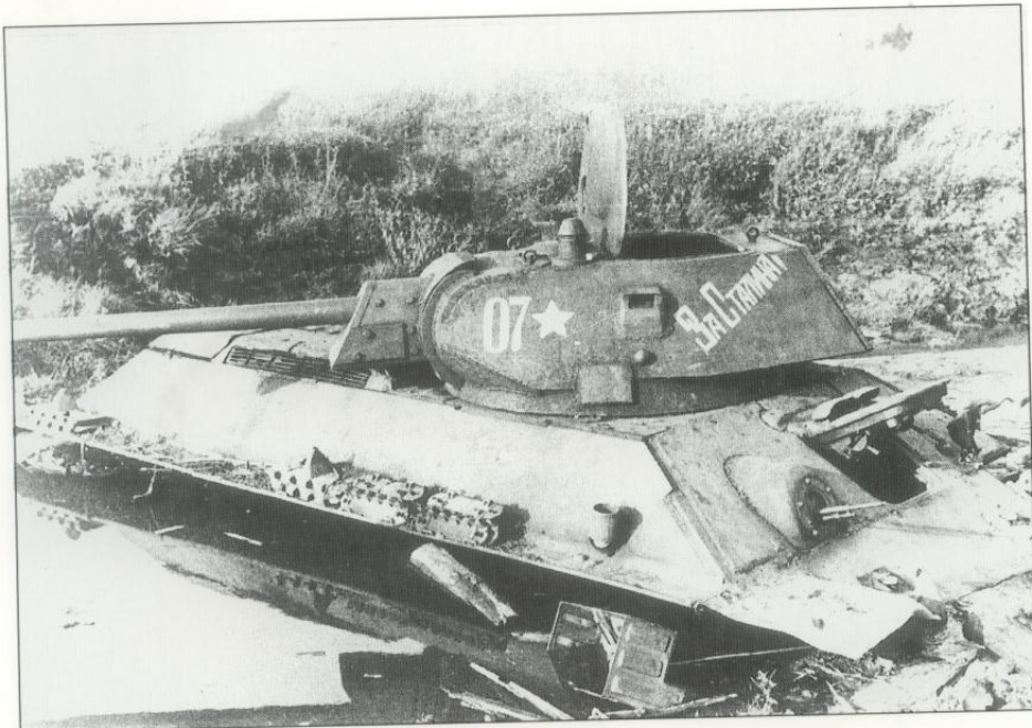
A T-34 Model 41/42 abandoned in a river during the summer of 1942. Note the features of this interim model produced at the Stalingrad Tractor Plant: the new pattern driver's hatch, the interlocked glacis armour, the chisel-shaped gun recuperator housing, the undercut turret front and the flat turret rear plate.
