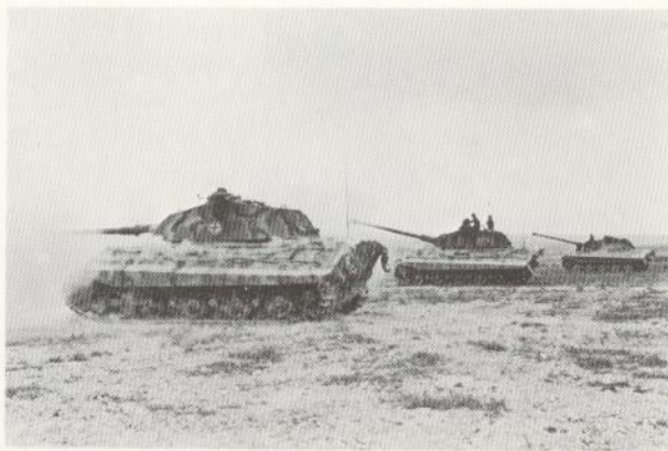
3/sPzAbt.503 'shooting in' their new Königstigers;note the heavy muzzle blast of the '88. The two tanks on the right have their guns locked in elevation while gunnery instructors discuss the results of their shooting with the crews. (Bundesarchiv)
