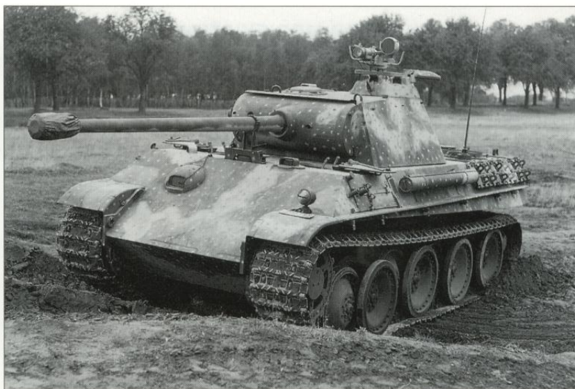
Starting late in 1944, some Panther Ausf.G were outfitted with the 'FG 1250' infra-red searchlight and scope. The FG 1250 was mounted on a rotating ring inside the upper lip in the commander's cupola. A steel band, threaded through a hole in the turret roof, connected the infra-red sensing scope to a device for sensing changes in the gun's elevation.
