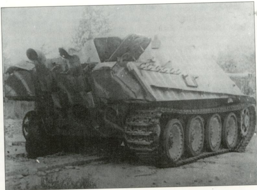
A rear view of one of the last Jagdpanther. This vehicle has the heating tower over the left fan outlet from the motor. The Flammvernichter (flame suppressor) on the exhaust pipes even have the hoods fitted.
