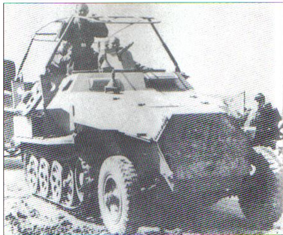
'Field mods' were common; this 251/7 Ausf. C engineers' half-track has been retro-fitted as a command vehicle with a salvaged aerial array from another type of AFV. Damaged mudguards were often removed, note the magnetic anti-tank mines - 'sticky bombs' - on the roof of this half-track.
