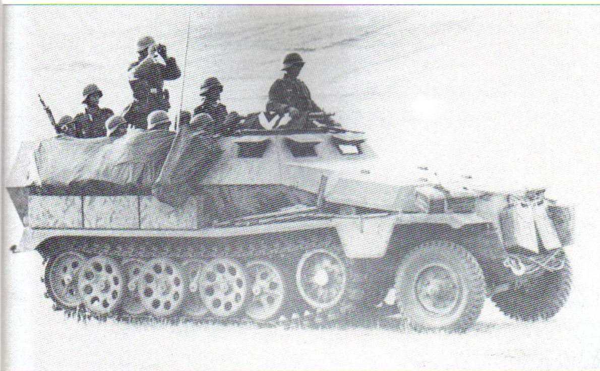
The slinging of jerrycans on the half-track emphasises the new flat one-piece nose plate of the Ausf. C; large armoured cowls protect the ventilators in the side of the engine compartment, and the exterior stowage bins are further back than on the Ausf. A and B.
