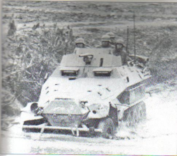
251/10 Ausf. A, bearing the 'inverted Y' sign which replaced the 1.Pz-Div.'s oakleaf for Operation 'Barbarossa', and fitted with an intermediate type of armoured shield for the PaK 36 3.7cm gun. The whole shield moved with the gun, and the side extensions gave added protection to the crew and commander.
