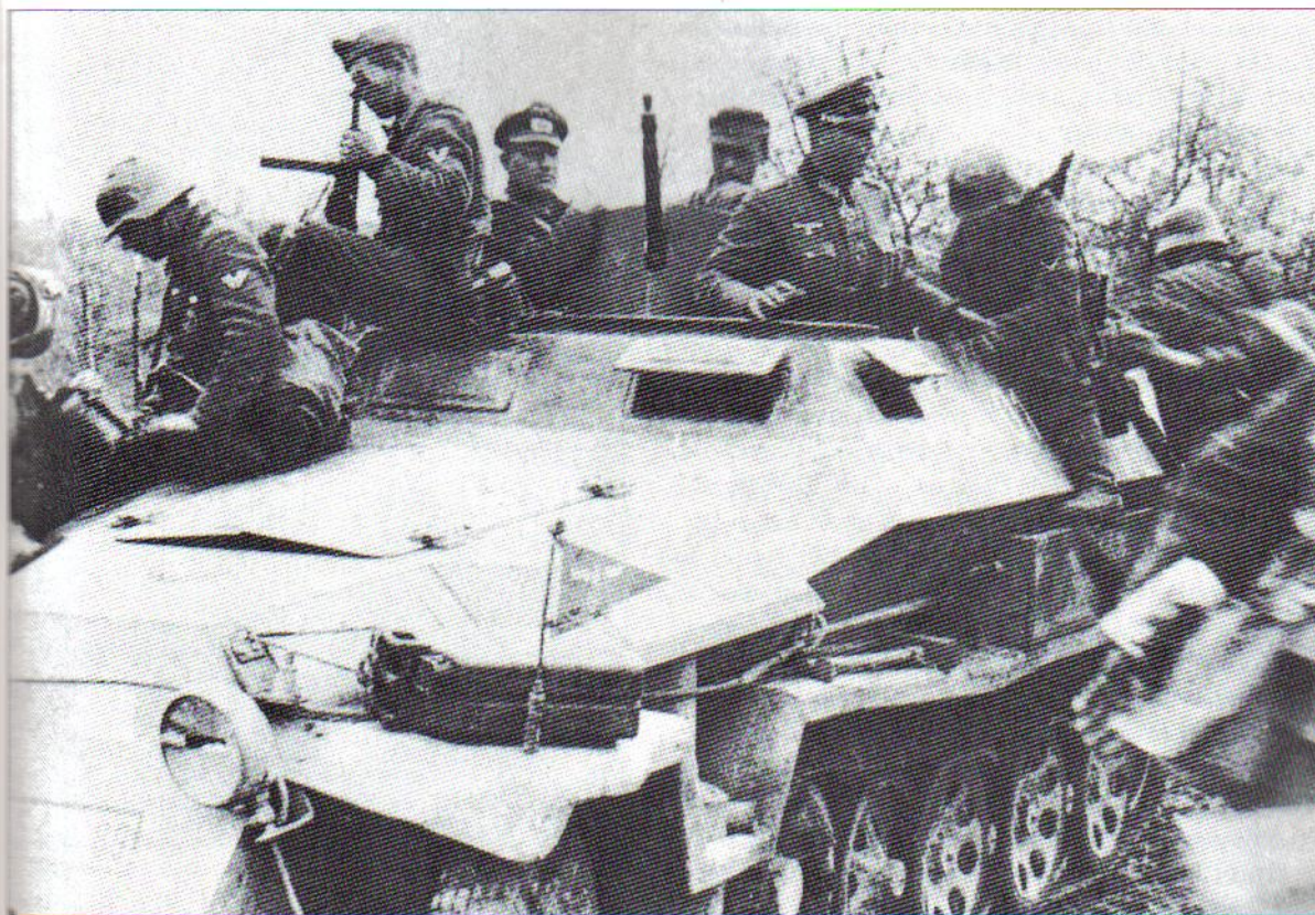
251/6 Ausf. C of Panzergrenadier-Regt. 'Grossdeutschland' commander, Oberst Lorenz, photographed in 1943; Lorenz is seen at right in vehicle, with goggles on service cap. Note the white divisional sign of 'GD' on the nose plate, the command flag in grey and white, and '01' on hull side.
