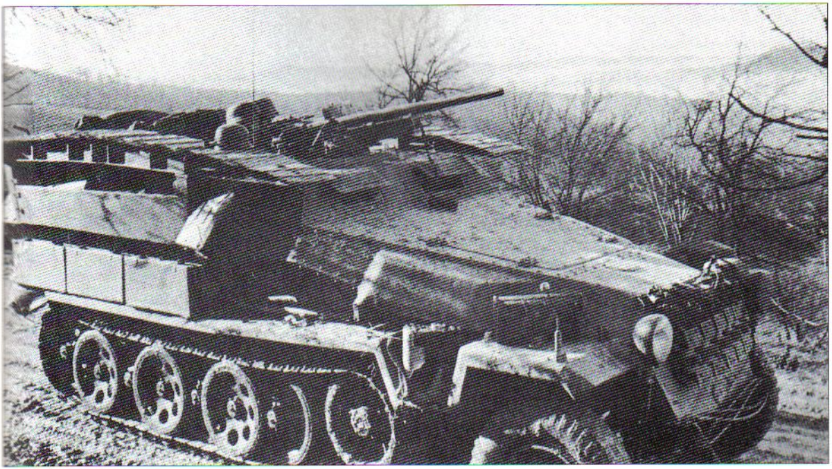
Ausf. C Pionierpanzerwagen fitted with a 3.7cm 'door-knocker' in place of the forward MG34.
