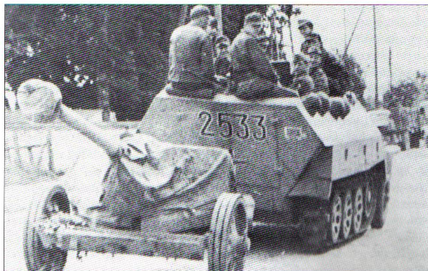
SdKfz 251/4 Ausf. D of 5.SS-Panzer-Division 'Wiking' towing a 7.5cm PaK40 anti-tank gun on the Eastern Front, 1944-45. The shortage of SP weapons in many units forced the retention of towed guns until the end of the war. The tactical sign on the right rear hull seems to indicate the motorised, rather than the armoured, battalion of this Panzergrenadier regiment, which must have been either 'Germania' or 'Westland' at this date. The divisional sign of a white 'mobile' swastika in circular form appears within a shield to the left of the white-trimmed black vehicle number '2533'.
