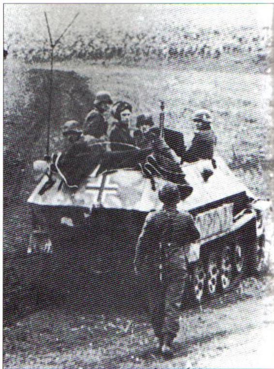
251 Ausf. C of an armoured infantry platoon of Panzergrenadier-Division 'Grossdeutschland' in action in Russia during September 1943, when the division was being ground down in fierce defensive fighting on the southern flank of the great Russian advance after the Kursk battles. Note cross on rear hull; prominent white divisional sign on door; 'crow's-foot' antenna; and three-colour camouflage paint scheme, in an obviously flamboyant pattern.
