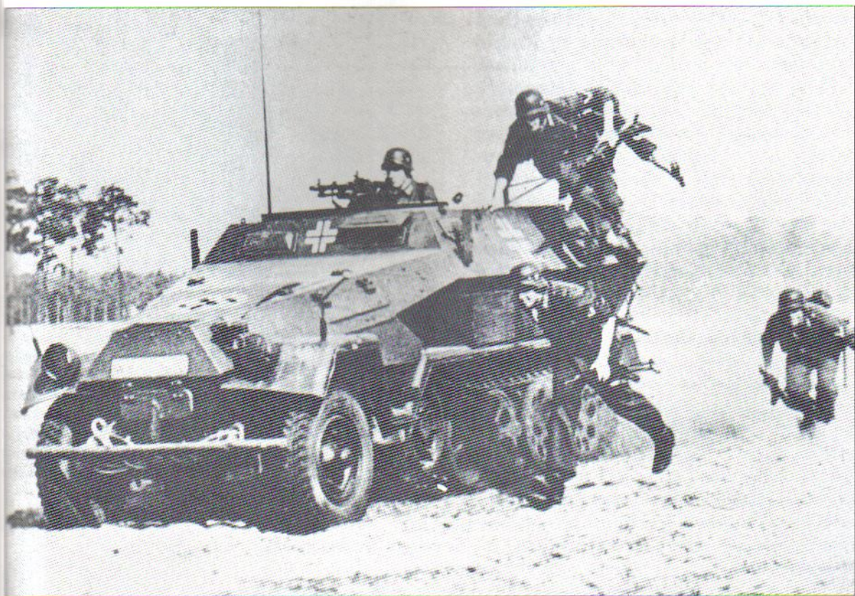
Classic photo of armoured infantry dismounting from an Ausf. B to deal with an obstacle. Note heavy front MG mount; and use of balkenkreuz marking between vision ports at front.
