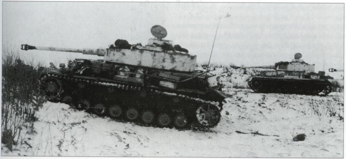
The combined weight of the L/48 and thicker frontal armour tended to overload the front suspension of the Ausf. H, keeping the leaf-springs permanently bowed. The effect of this can be seen on the nearest vehicle. Although retaining the turret girdles both vehicles have shed their side skirts, the mounting rails for which are clearly visible; the rail nearest the camera appears to be badly distorted. Note the new position of the aerial mounting. Russia, early 1943. (Bundesarchiv)
