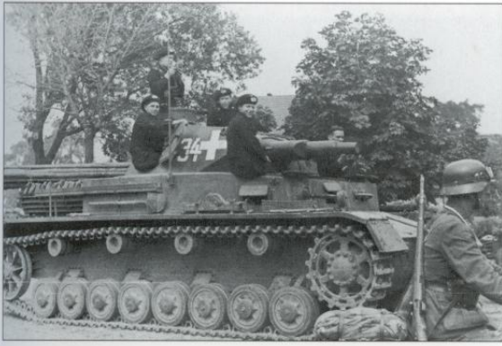
This Ausf. B probably belonged to the same unit and is identifiable by the straight front plate incorporating the hull machine-gun. The vehicle carries a small fascine for unditching purposes. See Plate A1. (Bundesarchiv)
