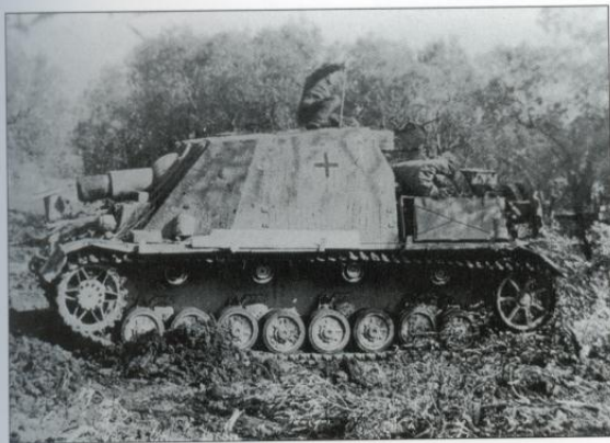
The massive construction of some buildings encountered during the street fighting in Stalingrad induced a demand for a heavy assault gun. The result was the Brumbär (Grizzly Bear), based on the PzKpfw chassis, which mounted a 150mm L/12 howitzer in a fixed superstructure. (US National Archives)
