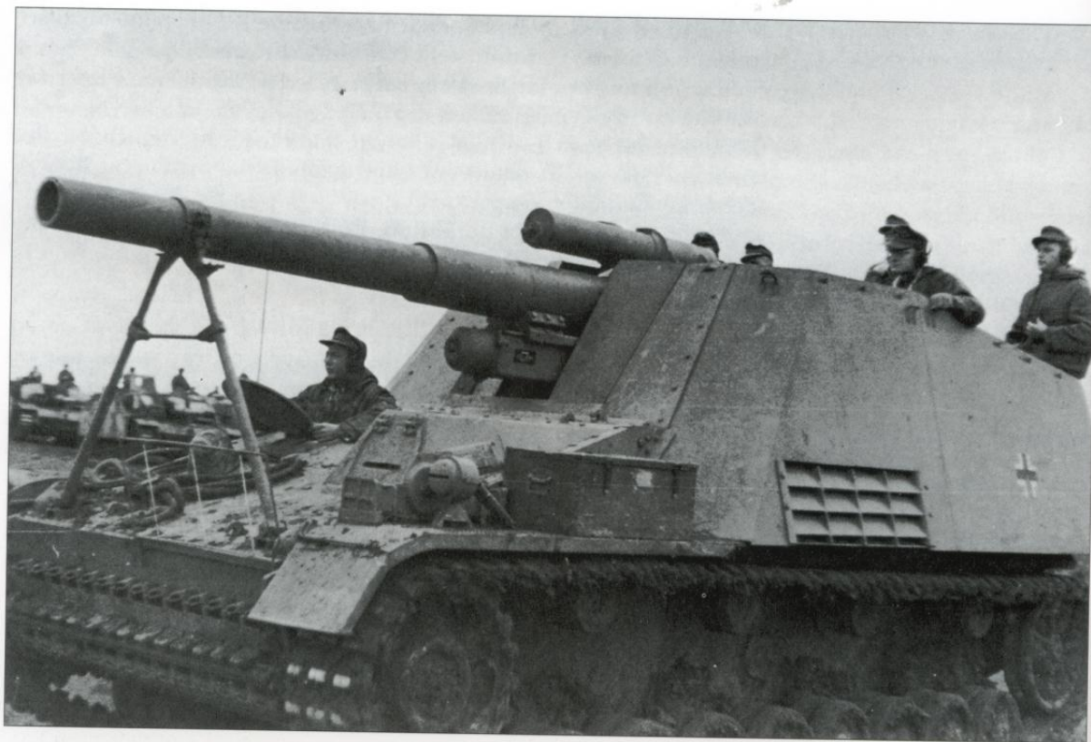
An early model of the 150mm SP howitzer Hummel (Bumble-bee), seen here on parade with an assault gun battalion. (Bundesarchiv)
